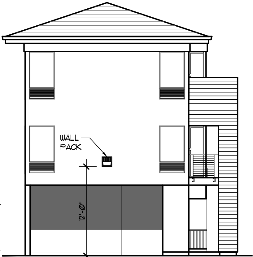
C FRONT ELEVATION SPR-8 SCALE : 1/8" = 1'-0"
