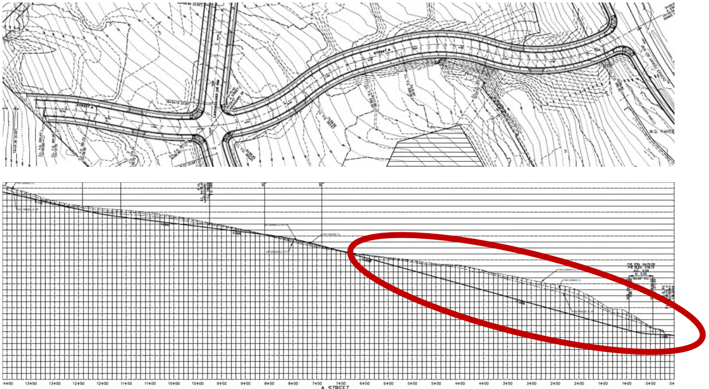
Figure 3: Plan view (top) and profile view (bottom) of the proposed A Street. This street is designed to "Collector B" standards and has been allowed to use Alternative Street Standards to have a street grade exceed 8%.
