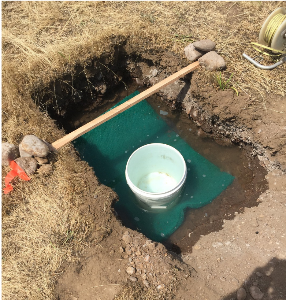
Photo A-1. Infiltration Test Pit for IT-1.
