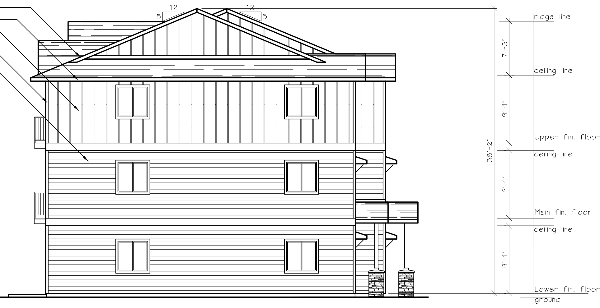
SOUTHWEST ELEVATION (TYPE A UNITS) SCALE: 1/8" = 1'-0" BLD. 7.8.10.24.28.+30
