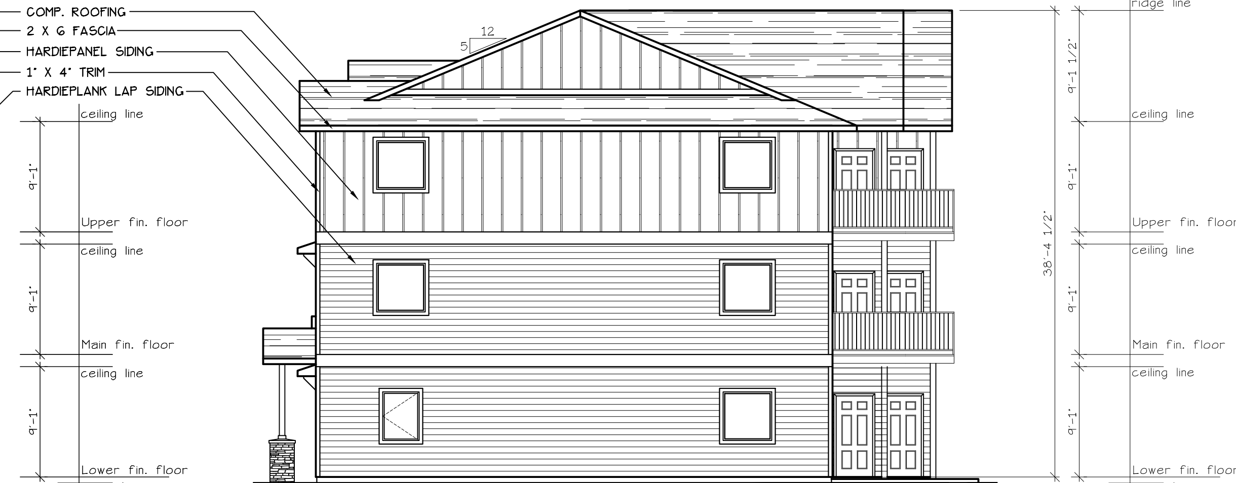
EAST ELEVATION (TYPE C UNITS) SCALE: 1/8" = 1'-0" BLD. 9.14.20.+33
