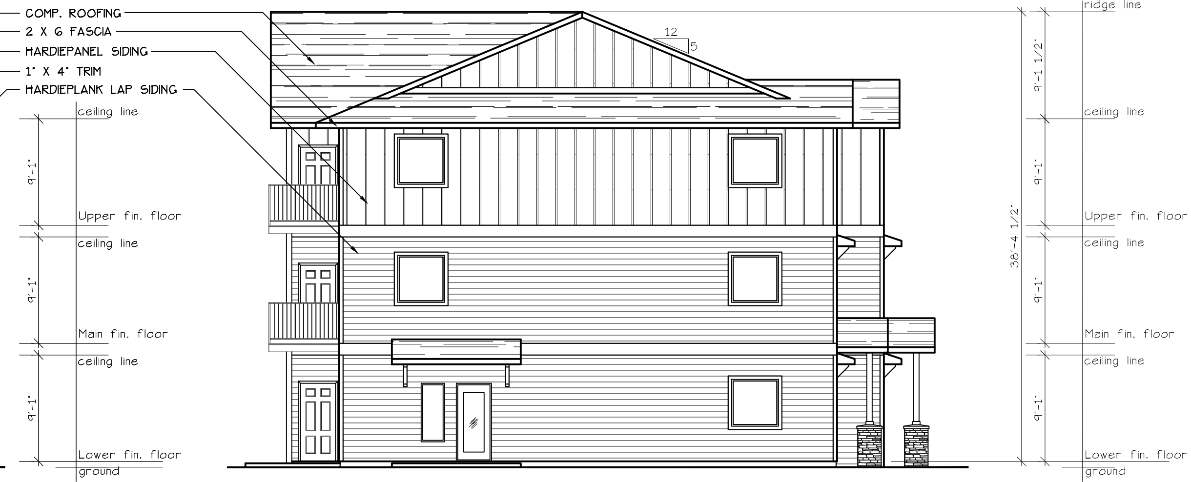
WEST ELEVATION (TYPE C UNITS) SCALE: 1/8" = 1'-0" BLD. 9.14.20.+33
