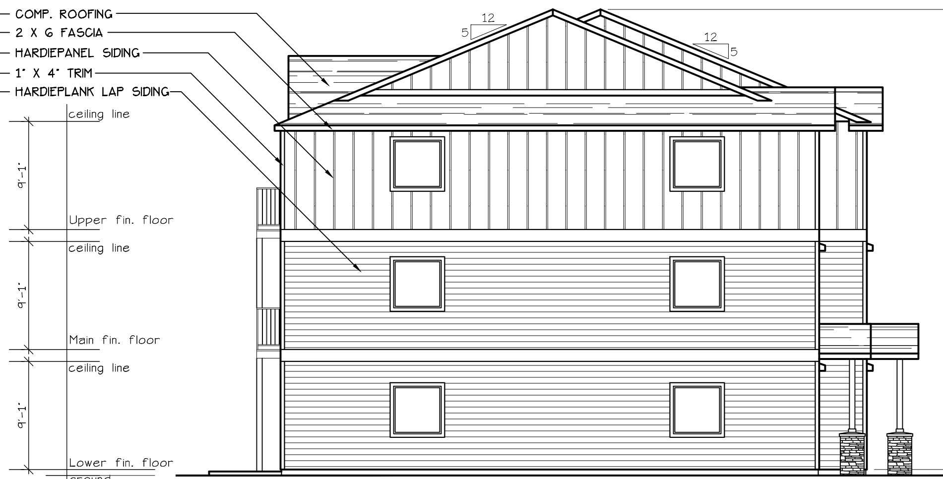
NORTH ELEVATION (TYPE B UNITS) SCALE: 1/8" = 1'-0" BLD. 13,19,23,26,+29
