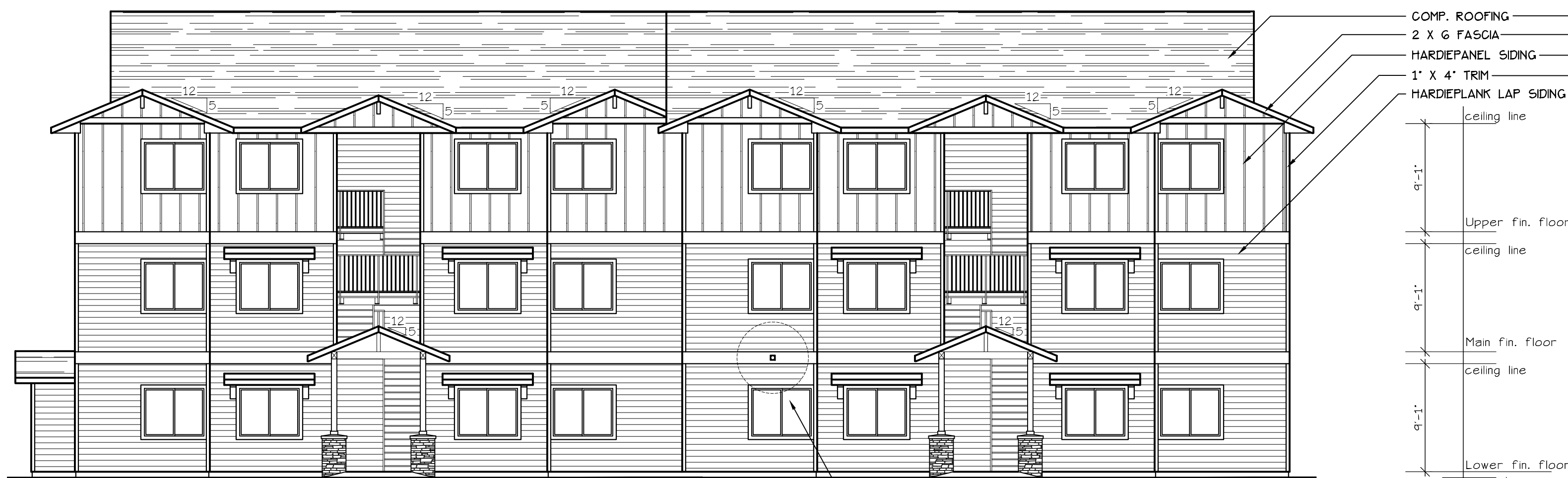
WEST ELEVATION (TYPE B UNITS) SCALE: 1/8" = 1'-0" BLD. 3 + 25
