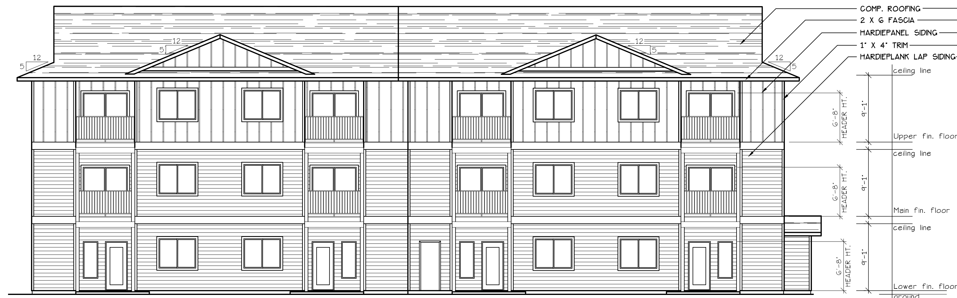
EAST ELEVATION (TYPE B UNITS) SCALE: 1/8" = 1'-0" BLD. 3 + 25
