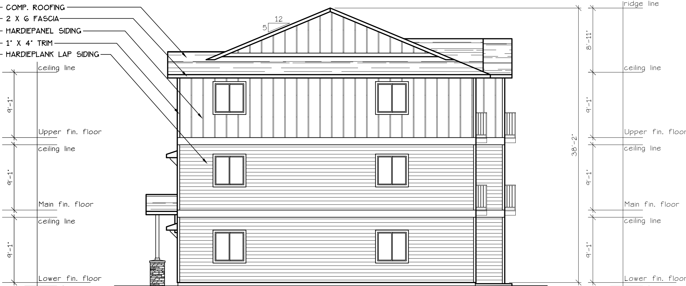
NORTHEAST ELEVATION (TYPE A UNITS) SCALE: 1/8" = 1'-0" BLD. 7.8.10.24.28.+30
