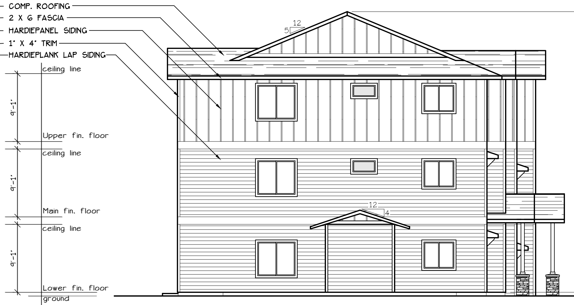
SOUTH ELEVATION (TYPE E UNITS) SCALE: 1/8" = 1'-0" BLD. 27
