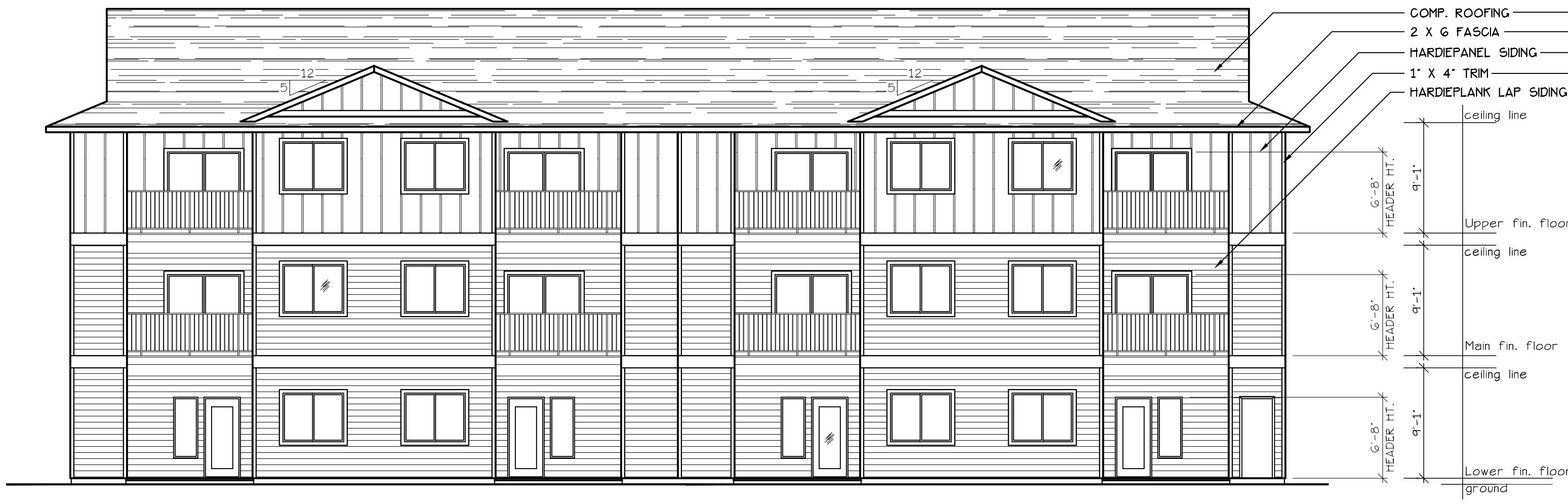
NORTHWEST ELEVATION (TYPE A UNITS) SCALE: 1/8" = 1'-0" BLD. 7.8.10.24.28.+30
