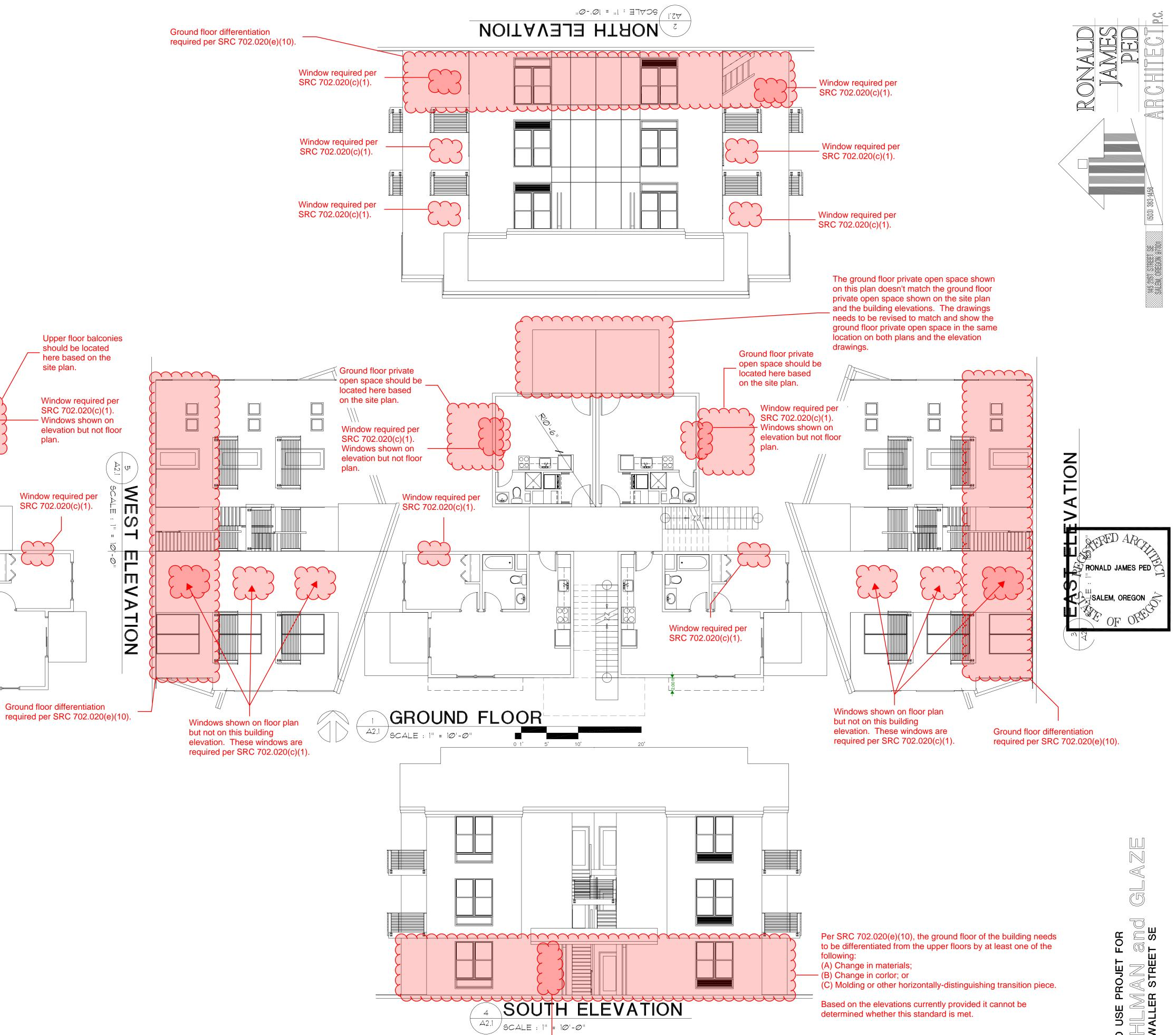
Entrance to this ground floor unit not shown on building elevation.
