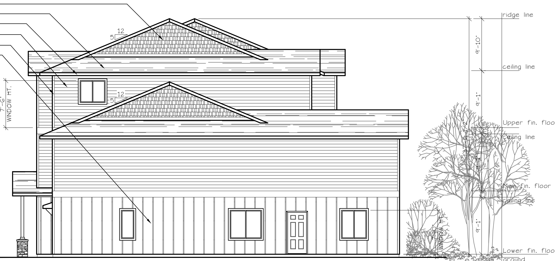
WEST ELEVATION (TYPE C UNITS) SCALE: 1/8" = 1'-0" BLD. 2
