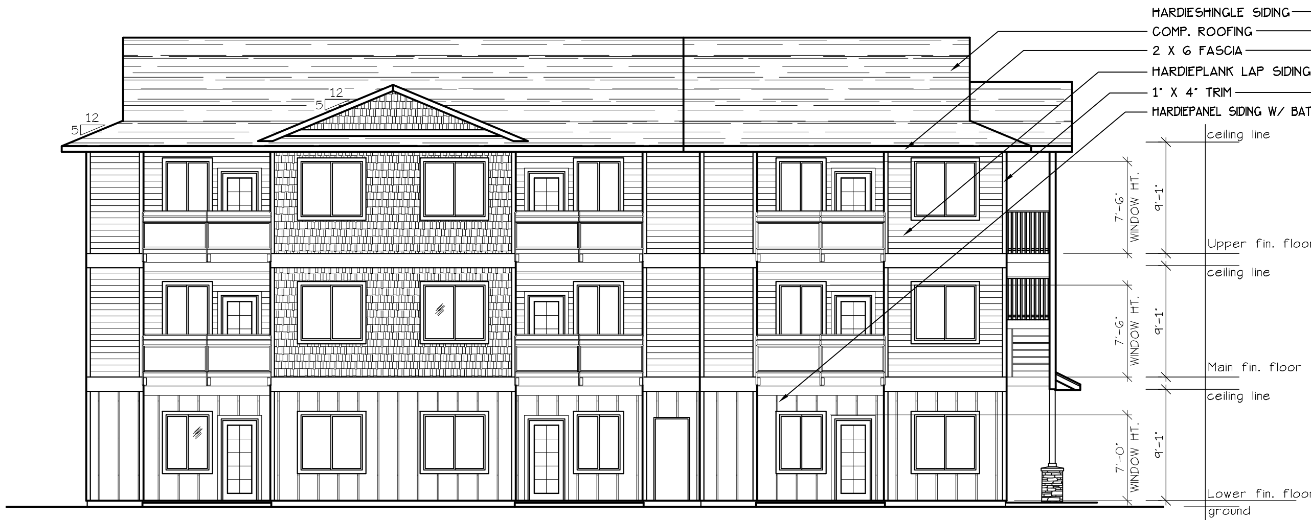
WEST ELEVATION (TYPE A UNITS) SCALE: 1/8" = 1'-0" BLD. 1
