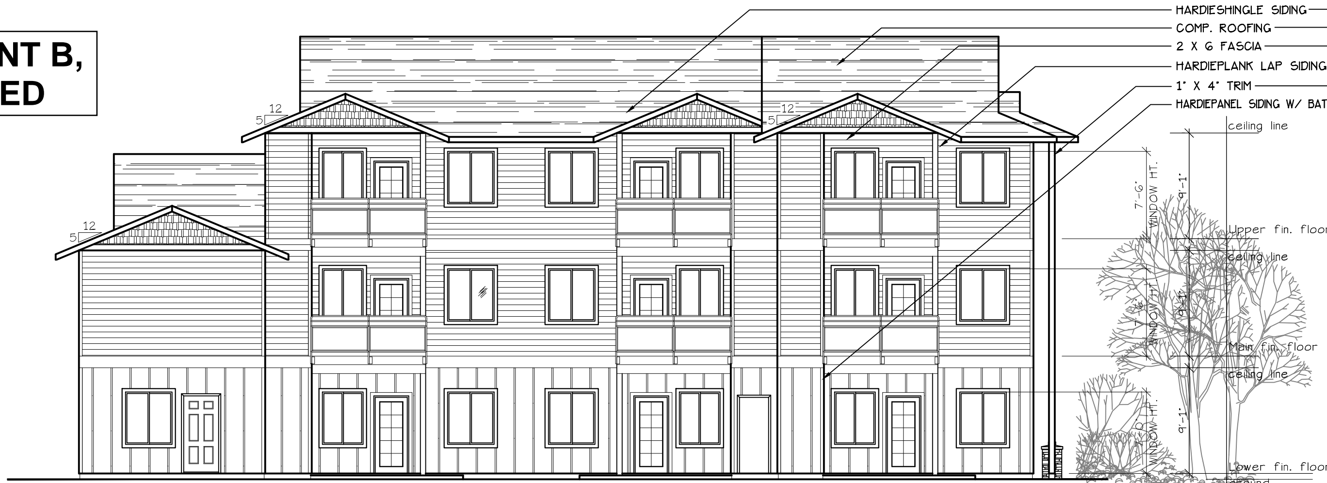
SOUTH ELEVATION (TYPE C UNITS) SCALE: 1/8" = 1'-0" BLD. 2
