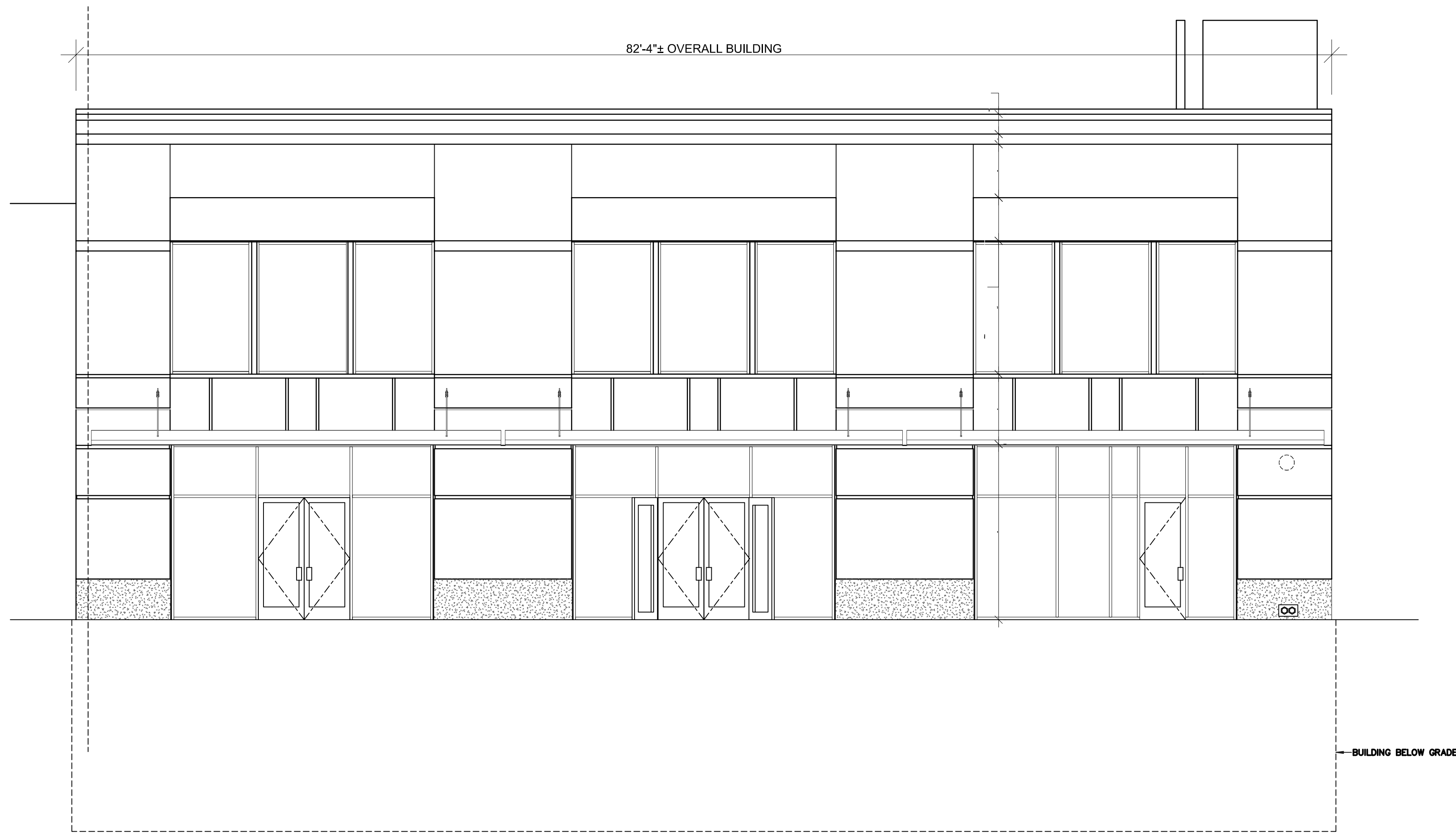
3 A4 EXISTING WEST ELEVATION - NO CHANGES 3/16" = 1' - 0"
