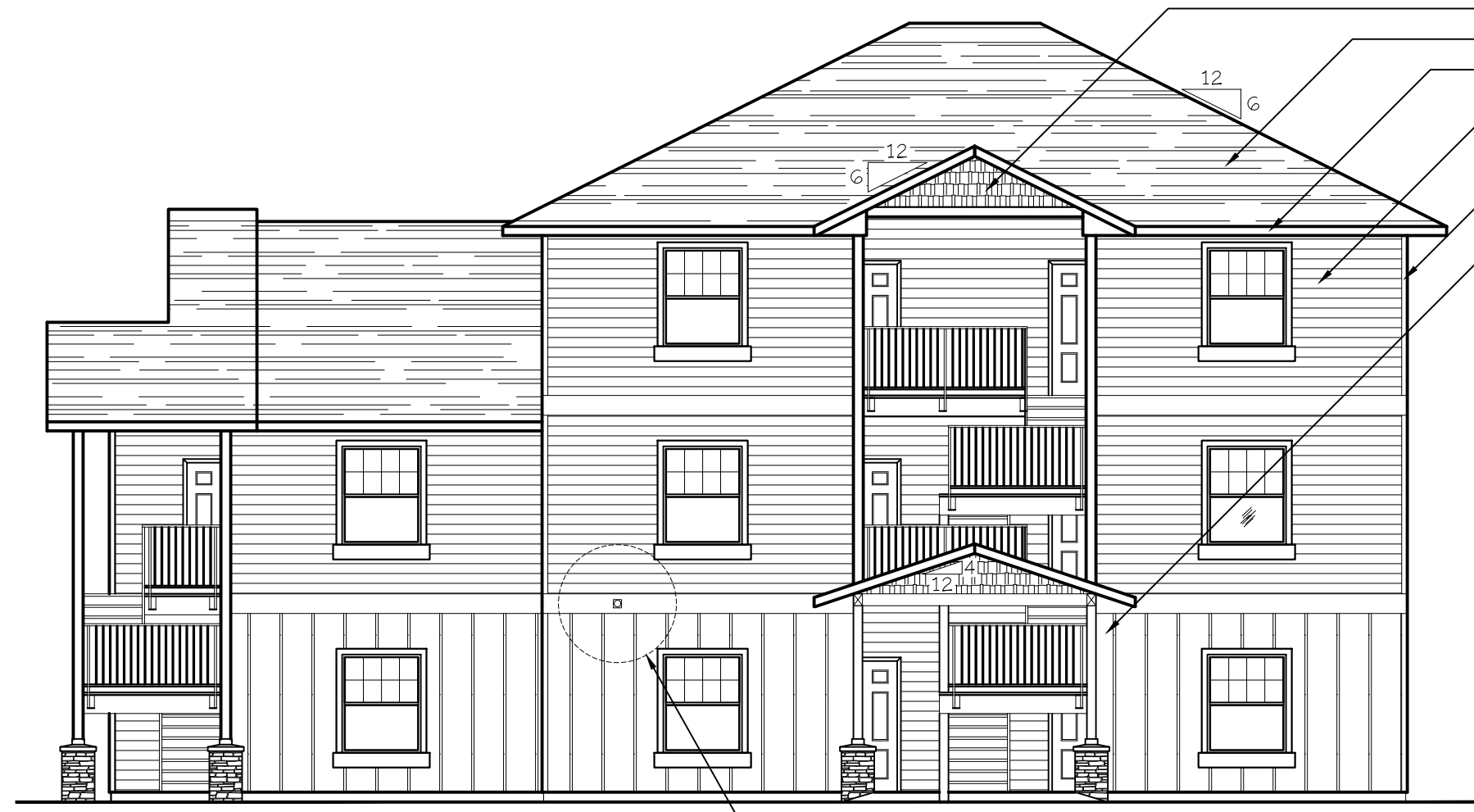
NORTH ELEVATION (TYPE C UNITS) SCALE: 1/8" = 1'-0" BLD. 17
