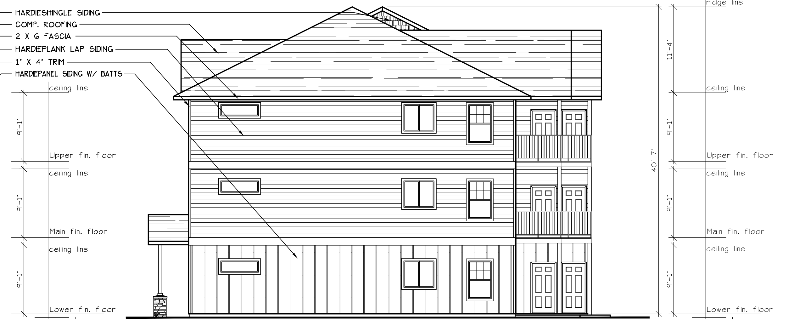
NORTH ELEVATION (TYPE G UNITS) SCALE: 1/8" = 1'-0" BLD. 2.7.9-12+15
