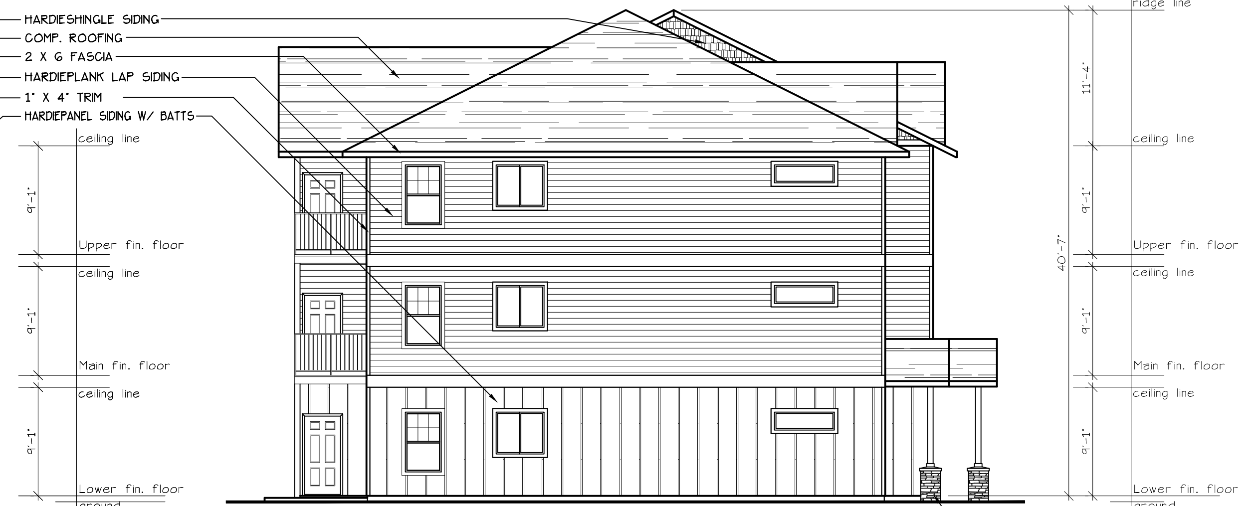
SOUTH ELEVATION (TYPE G UNITS) SCALE: 1/8" = 1'-0" BLD. 2.7.9-12+15
