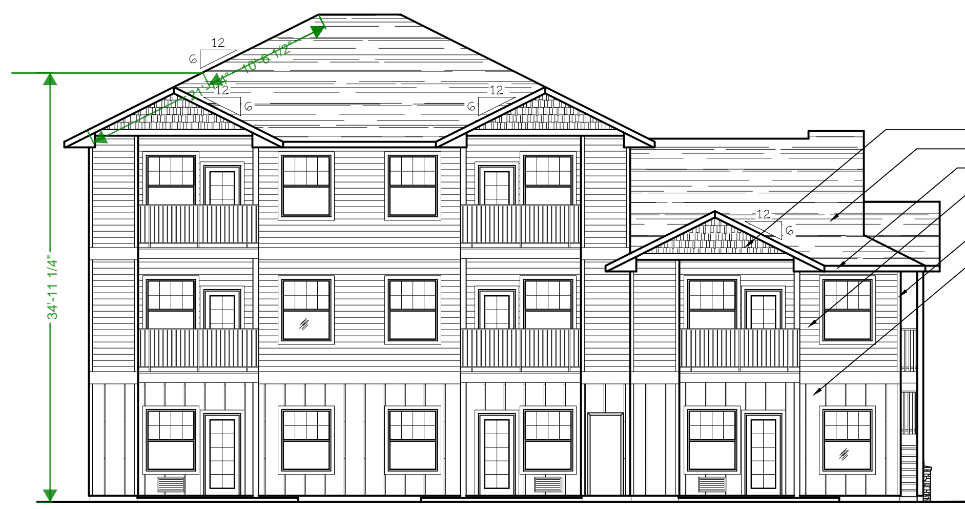
SOUTH ELEVATION (TYPE C UNITS) SCALE: 1/8" = 1'-0" BLD. 17
