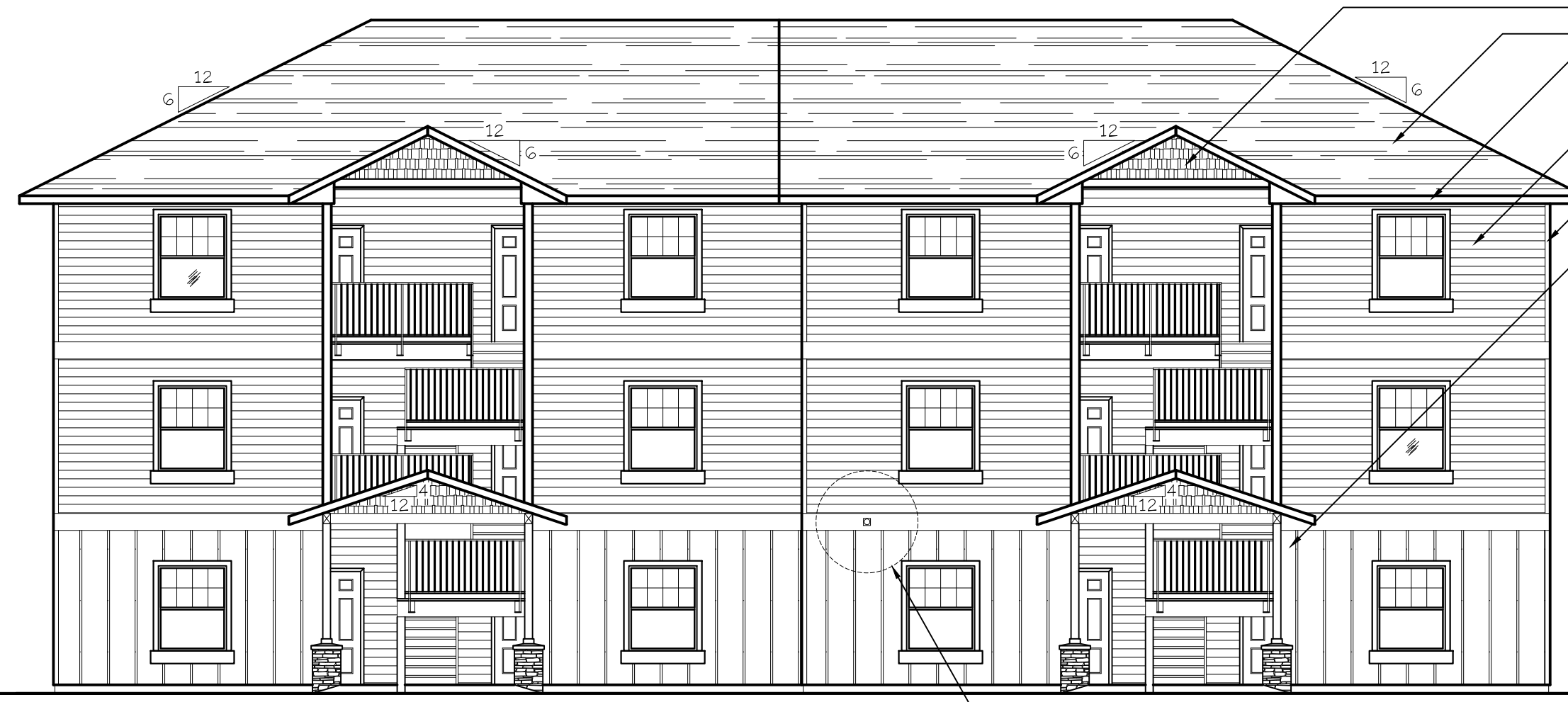
WEST ELEVATION (TYPE C UNITS) SCALE: 1/8" = 1'-0" (BLD. 1+3)
