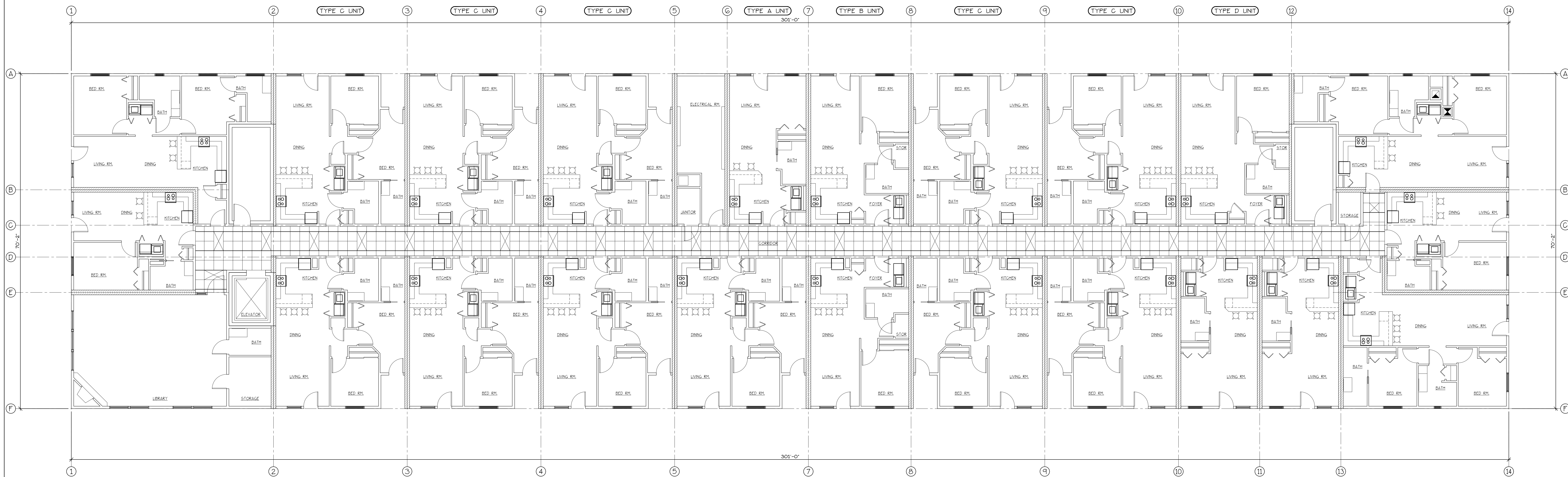
SECOND FLOOR SUSPENDED CEILING PLAN
