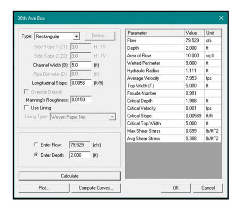
The box culvert has also been analyzed to ensure that it has adequate capacity to convey the 50-year storm at full build-out conditions. Flows were taken from West Consultants' model provided in the Pringle Creek Basin Master Plan. The conveyance capacity of the culvert for the 50-year storm event can be seen below.
