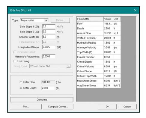
Flows for the 50-year storm event were taken from West Consultants' model provided in the Pringle Creek Basin Master Plan. The conveyance capacity of the ditch for the 50-year storm event can be seen below.
