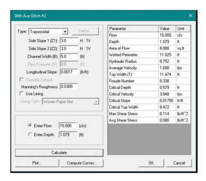
As can be seen from the analysis, the ditches along the West side of 36<sup>th</sup> Avenue has more than adequate capacity to convey the proposed buildout conditions.
