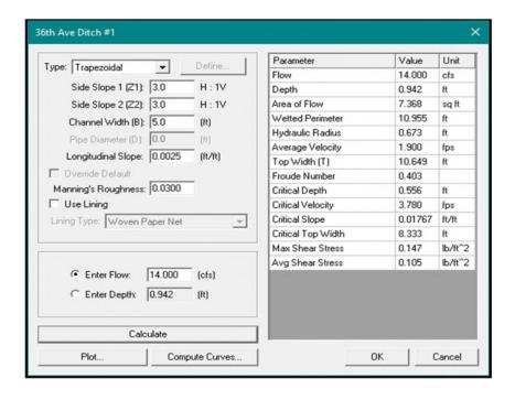
As can be seen from the analysis Ditch #1 has more than adequate capacity to convey the 50-year storm event at full buildout conditions, as required by the City of Salem Standards for arterials. Ditch #2 was also analyzed for the full flow capacity and the ability to convey the 50-year storm event. The results can be seen below.
