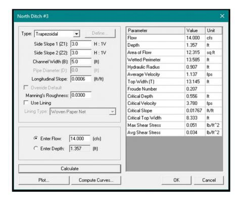
As can be seen from the above analysis, the ditch system along Boone Road will have more than adequate capacity to convey the 50-year event at full buildout conditions.
