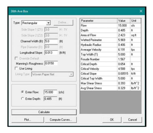
Per this analysis, the box culvert at the crossing of 32<sup>nd</sup> and 36<sup>th</sup> Avenue will have more than adequate capacity to convey the full build-out conditions.
