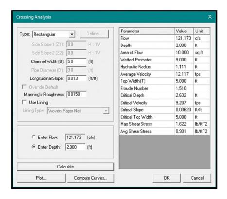
The culvert was also analyzed for the 50-year storm event. Flows were taken from West Consultants' model provided in the Pringle Creek Basin Master Plan. The conveyance capacity of the culvert for the 50-year storm event can be seen below.
