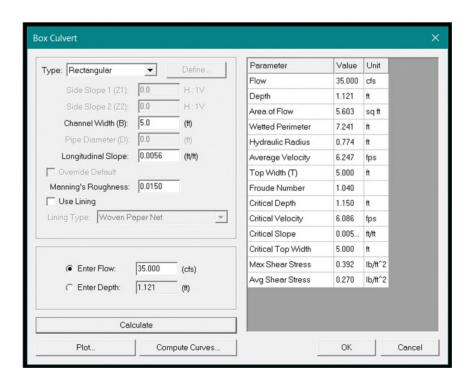
The improved box culvert at the crossing of Boone Road and 36<sup>th</sup> Avenue will have adequate capacity to convey the full buildout 50-year storm event based on the above analysis.
