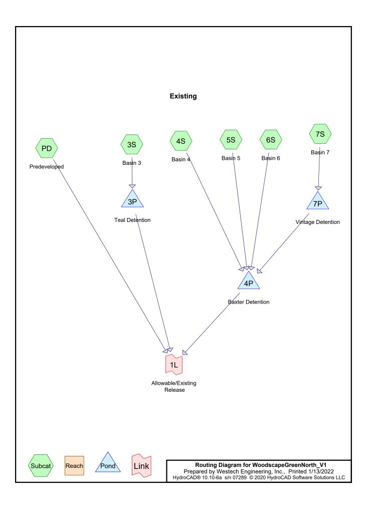
HydroCAD® 10.10-6a s/n 07289 © 2020 HydroCAD Software Solutions LLC
