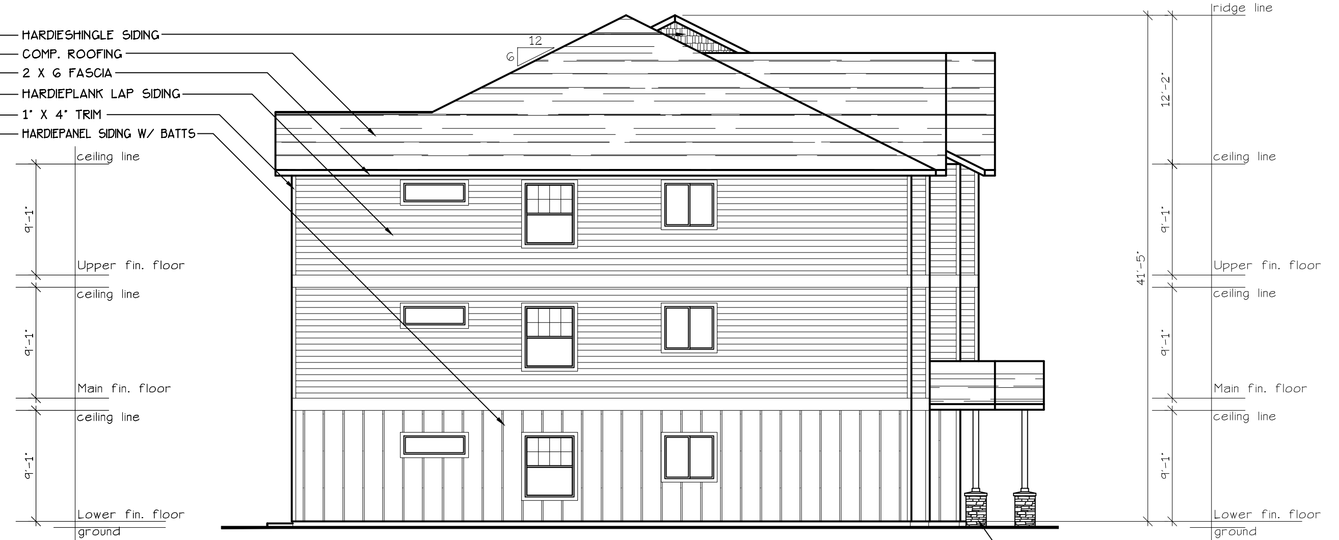
SOUTH ELEVATION (TYPE F UNITS) SCALE: 1/8" = 1'-0" BLD. 14
