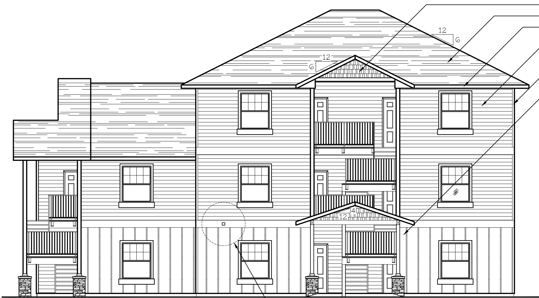
NORTH ELEVATION (TYPE C UNITS) SCALE: 1/8" = 1'-0" BLD. 17 EXHAUST VENT 3'-0" CLEAR OF OPERABLE WINDOW AREA TYP.
