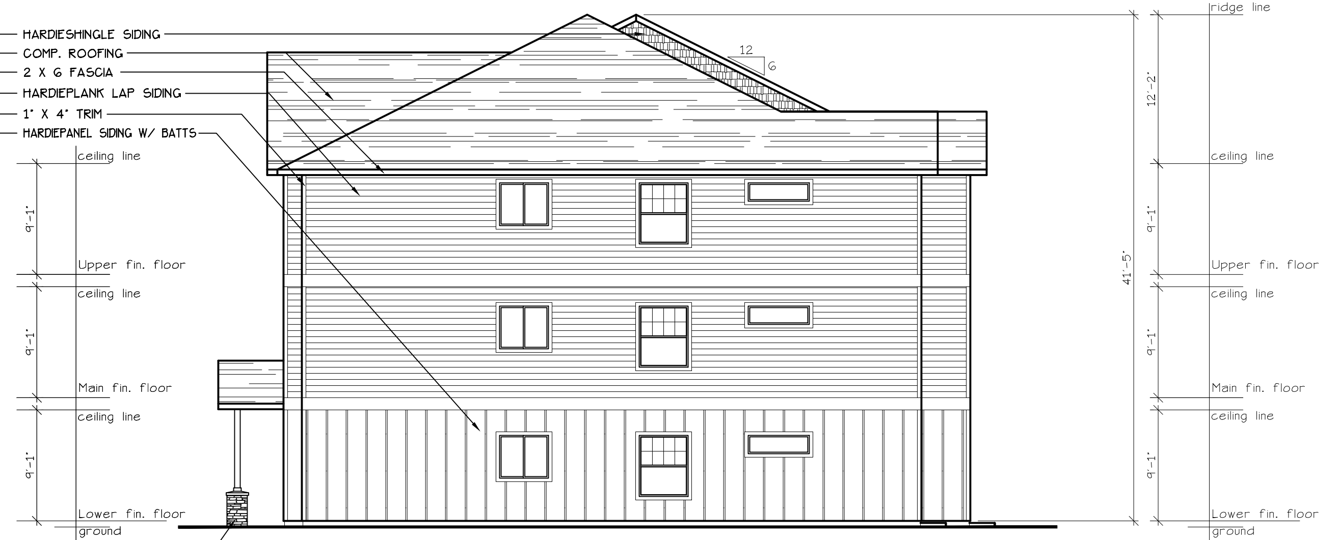
NORTH ELEVATION (TYPE F UNITS) SCALE: 1/8" = 1'-0" BLD. 14
