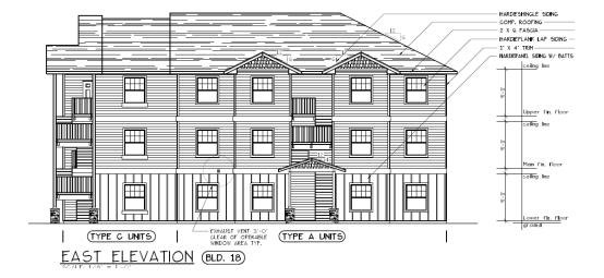
The proposed buildings proved the required offsets and design elements as shown on the building elevations.
