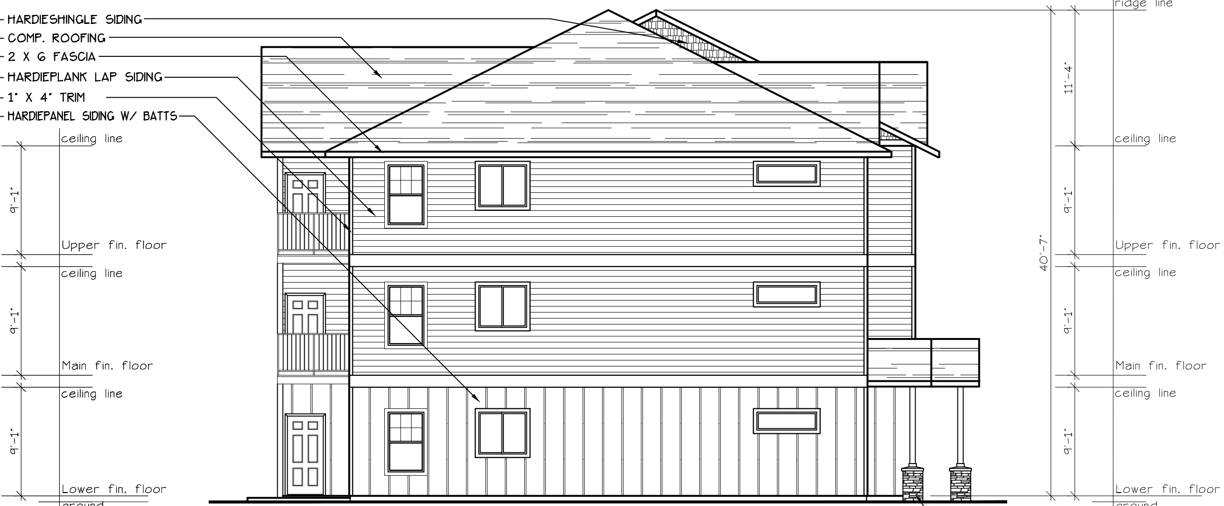
SOUTH ELEVATION (TYPE G UNITS) SCALE: 1/8" = 1'-0" BLD. 2,7,9-12+15
