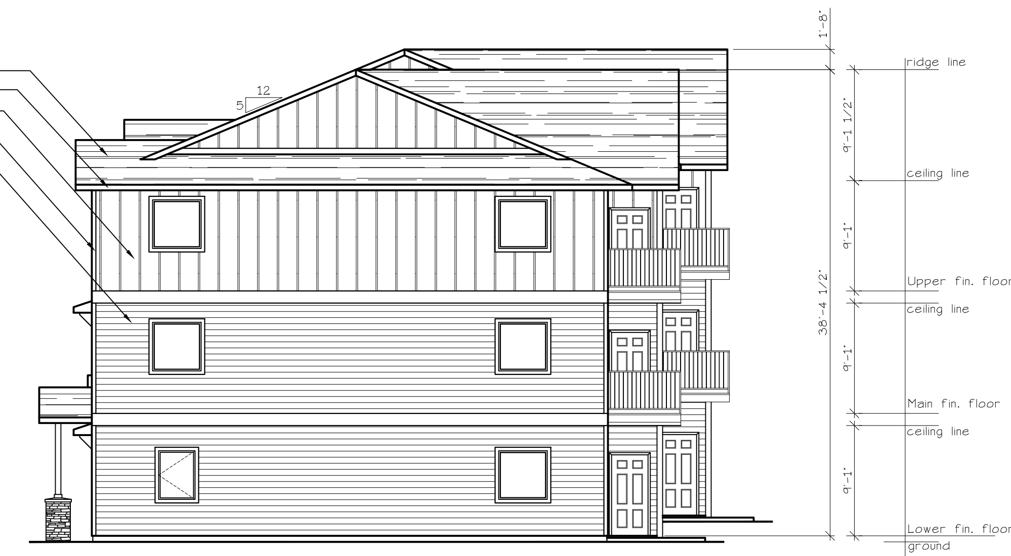
EAST ELEVATION (TYPE C UNITS) SCALE: 1/8" = 1'-0" BLD. 2
