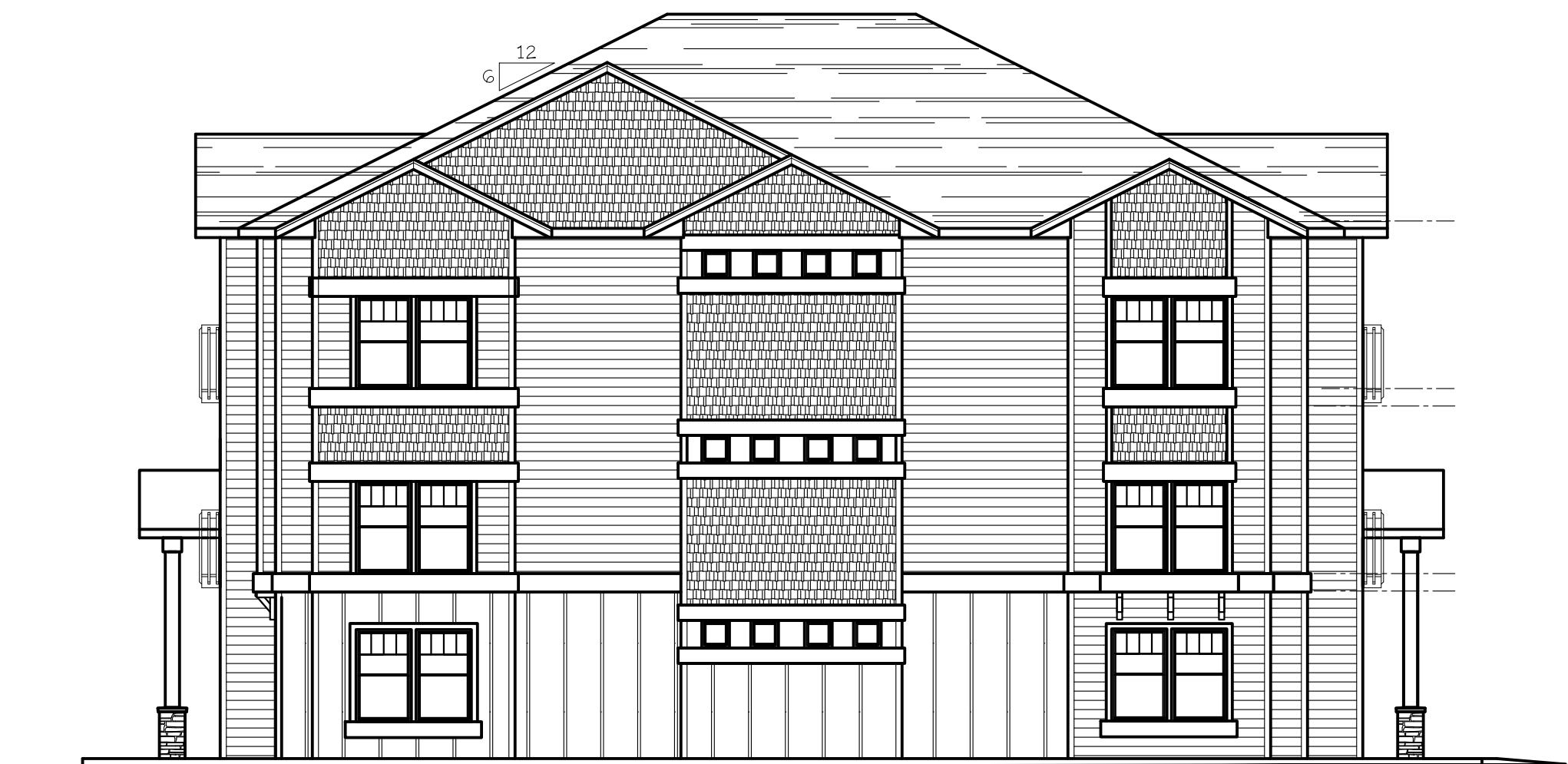
WEST ELEVATION (BLD. 27+31) SCALE: 1/8" = 1'-0" (TYPE E UNIT)
