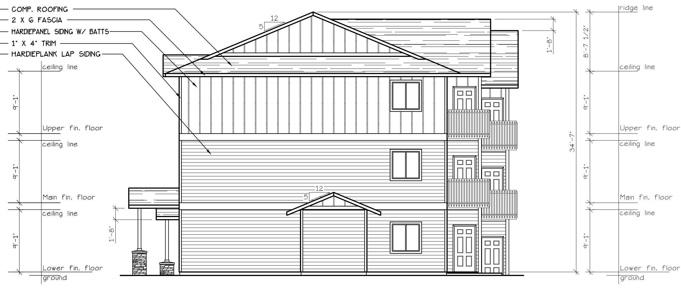
SOUTH ELEVATION (TYPE D UNITS) SCALE: 1/8" = 1'-0" BLD. 5
