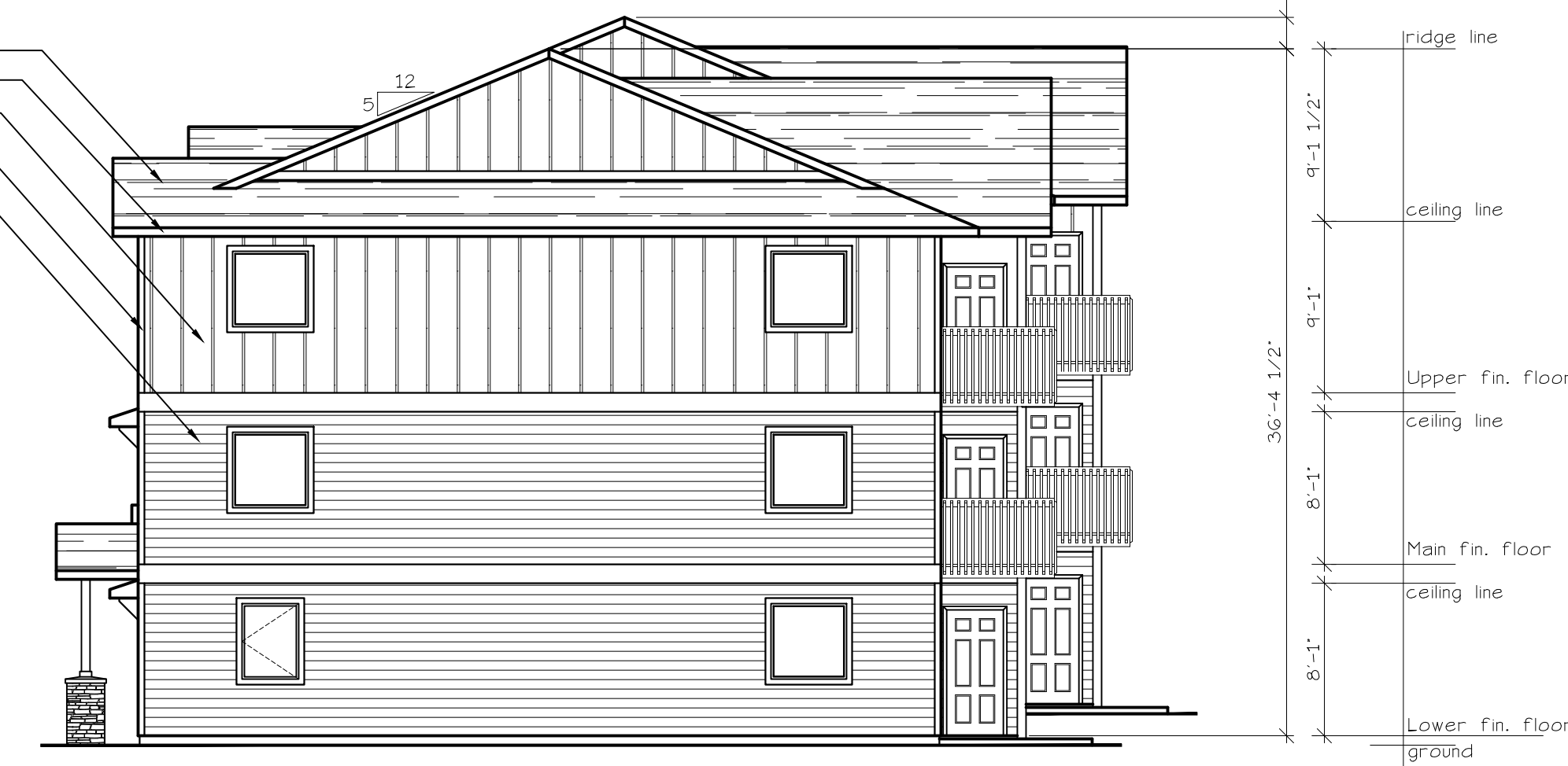
EAST ELEVATION (TYPE C UNITS) SCALE: 1/8" = 1'-0" BLD. 2
