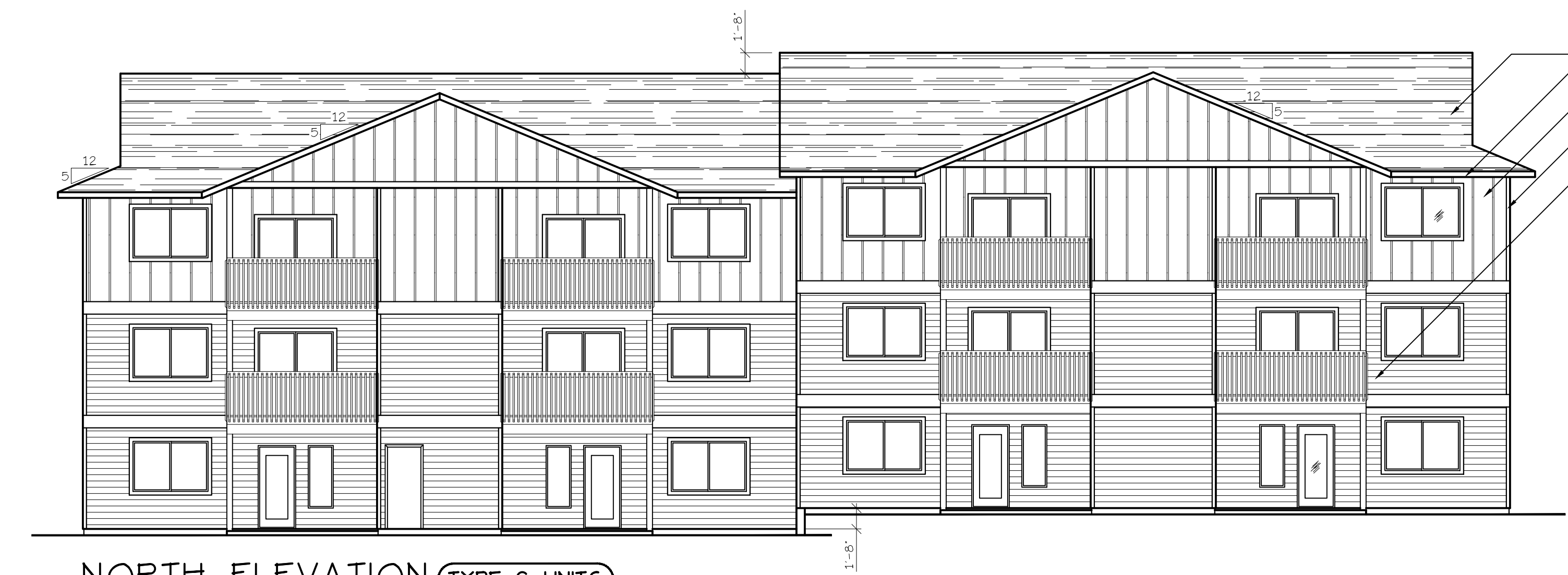
NORTH ELEVATION (TYPE C UNITS) SCALE: 1/8" = 1'-0" BLD. 2
