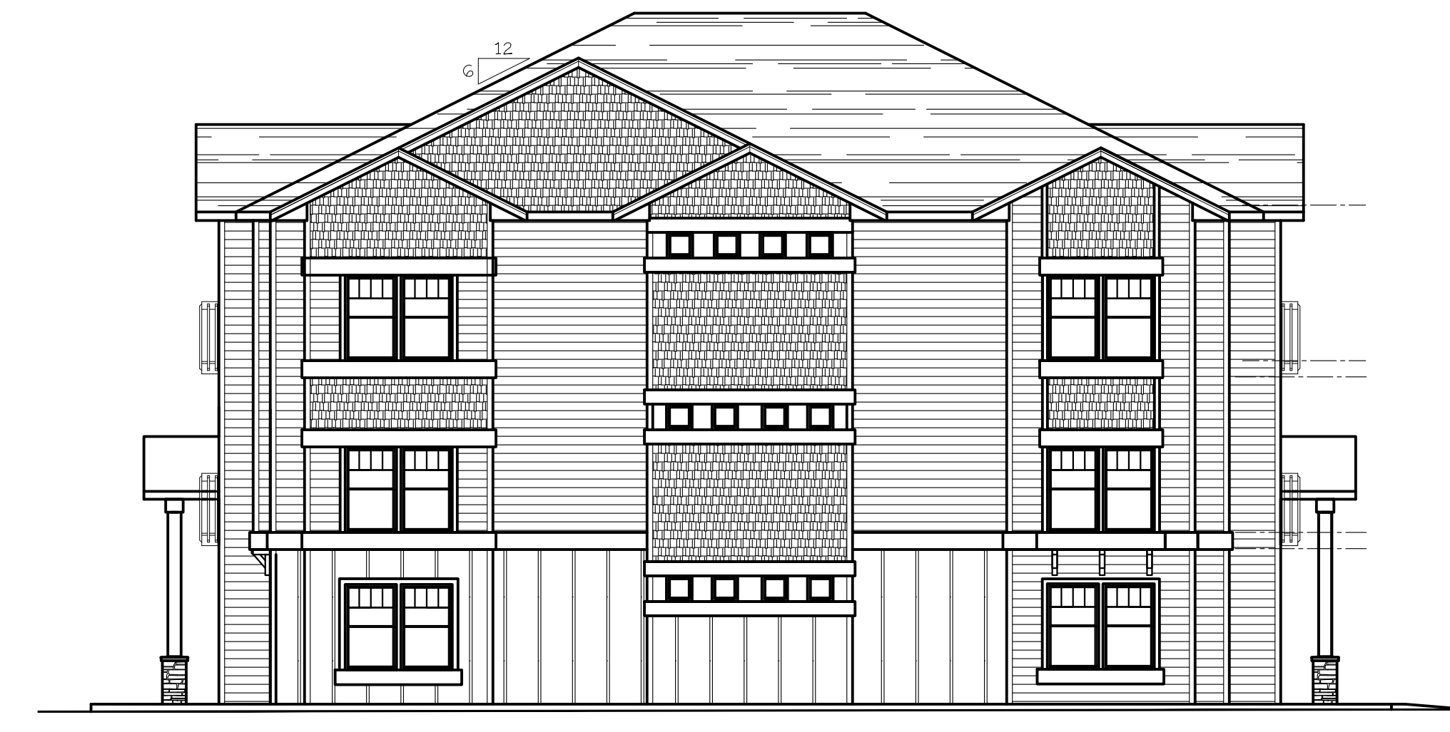
WEST ELEVATION (BLD. 27+31) SCALE: 1/8" = 1'-0" TYPE E UNIT
