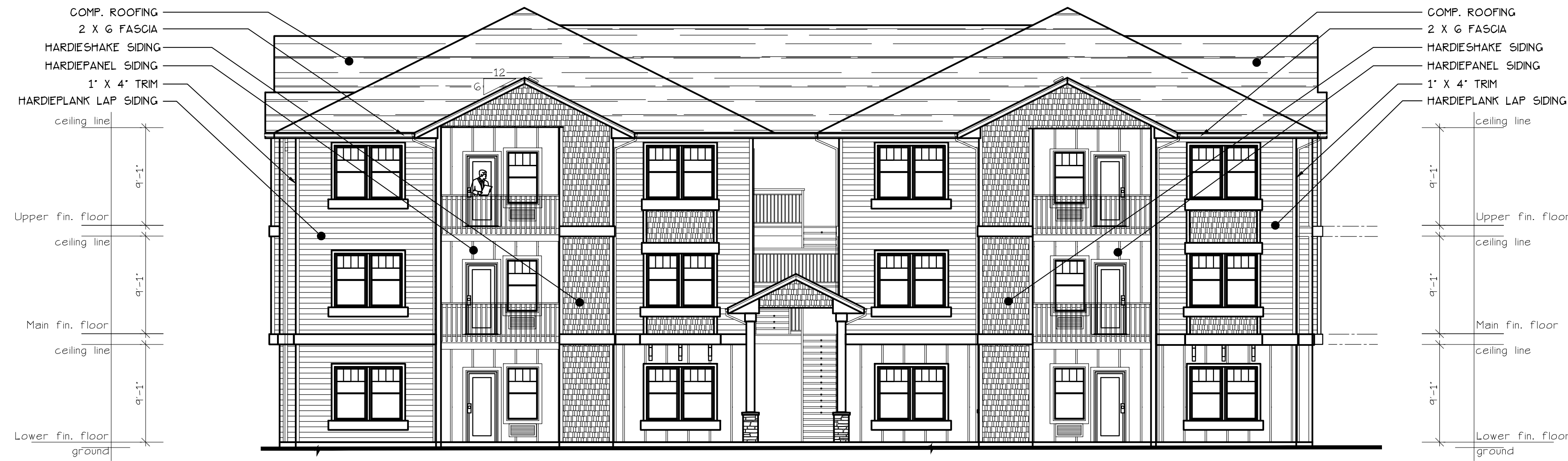
SOUTH ELEVATION (BLD. 27+31) SCALE: 1/8" = 1'-0" TYPE E UNIT
