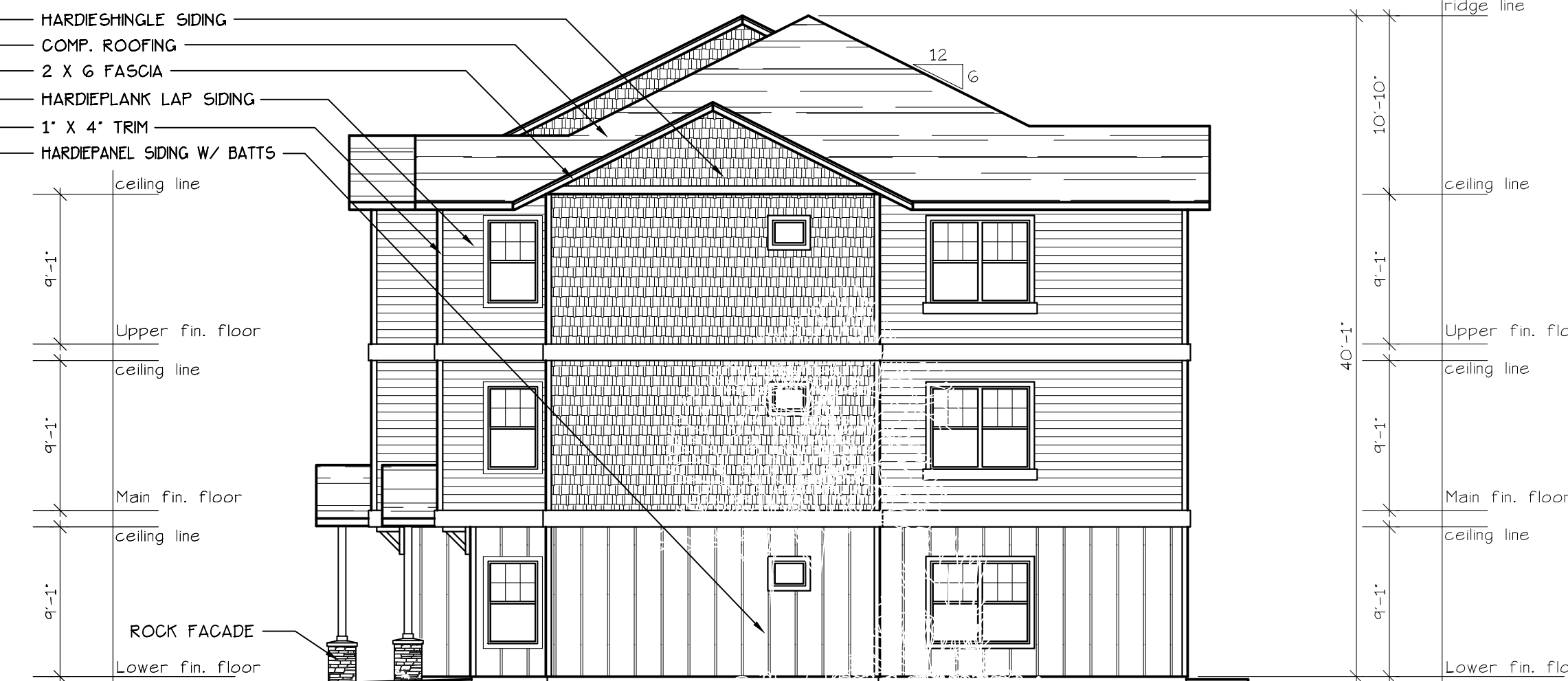
END ELEVATION (TYPE A UNITS) SCALE: 1/8" = 1'-0" BLD. 21+29
