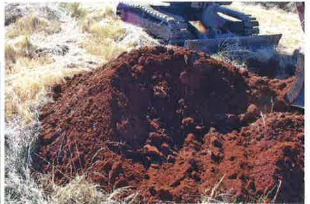
Decomposed Sentinel Bluff basalt spoils from test pit TP-1
