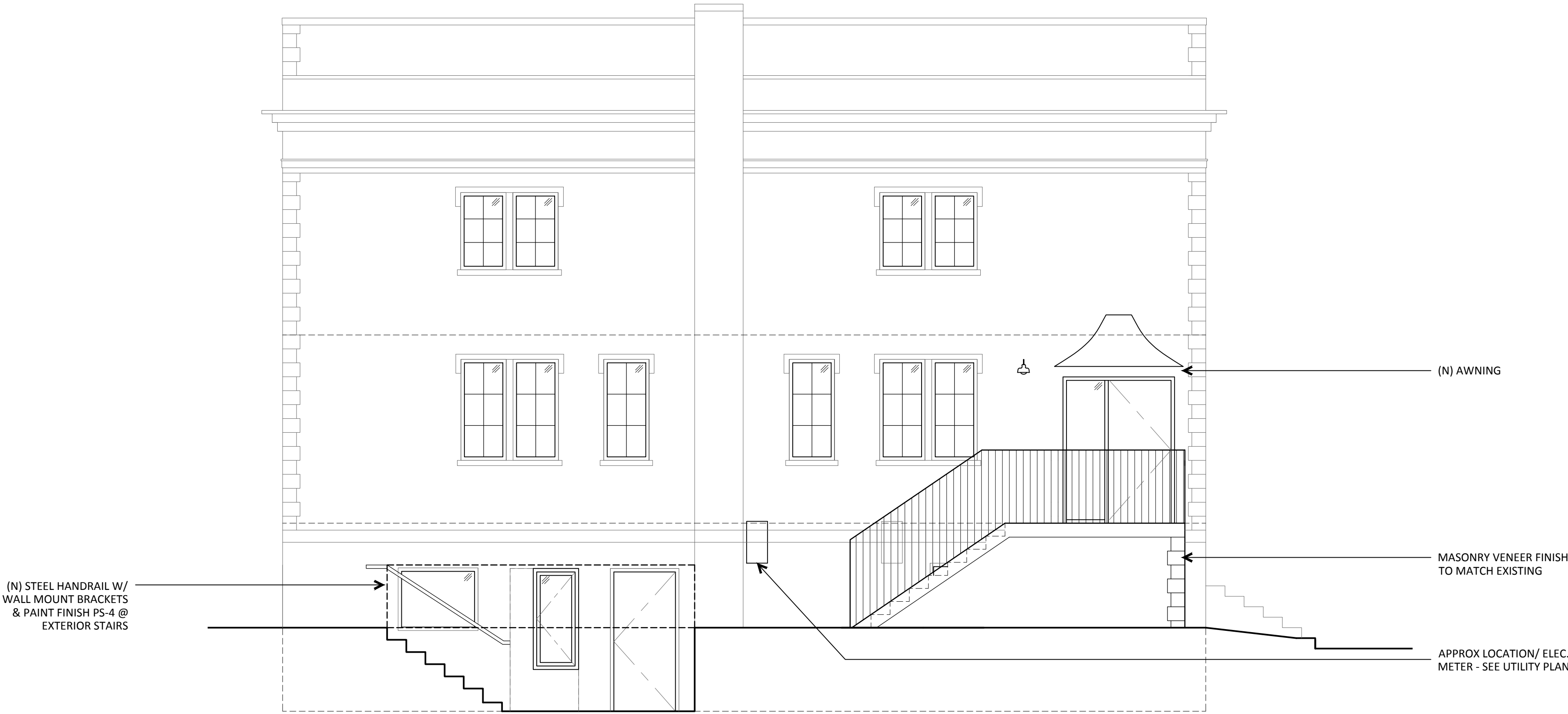
2 BUILDING "A" ELEVATION - WEST 1/4" = 1'-0"
