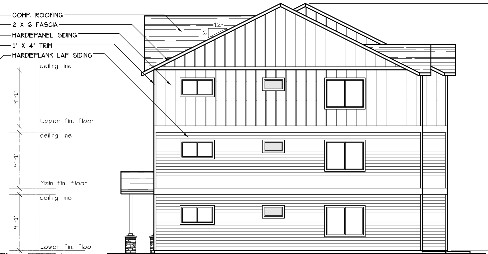
SOUTH ELEVATION (TYPE A UNITS) SCALE: 1/8" = 1'-0" BLD. 3
