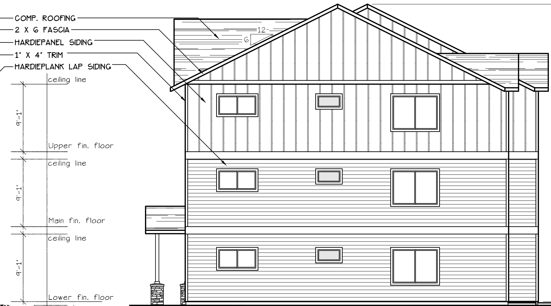
SOUTH ELEVATION (TYPE A UNITS) SCALE: 1/8" = 1'-0" BLD. 3
