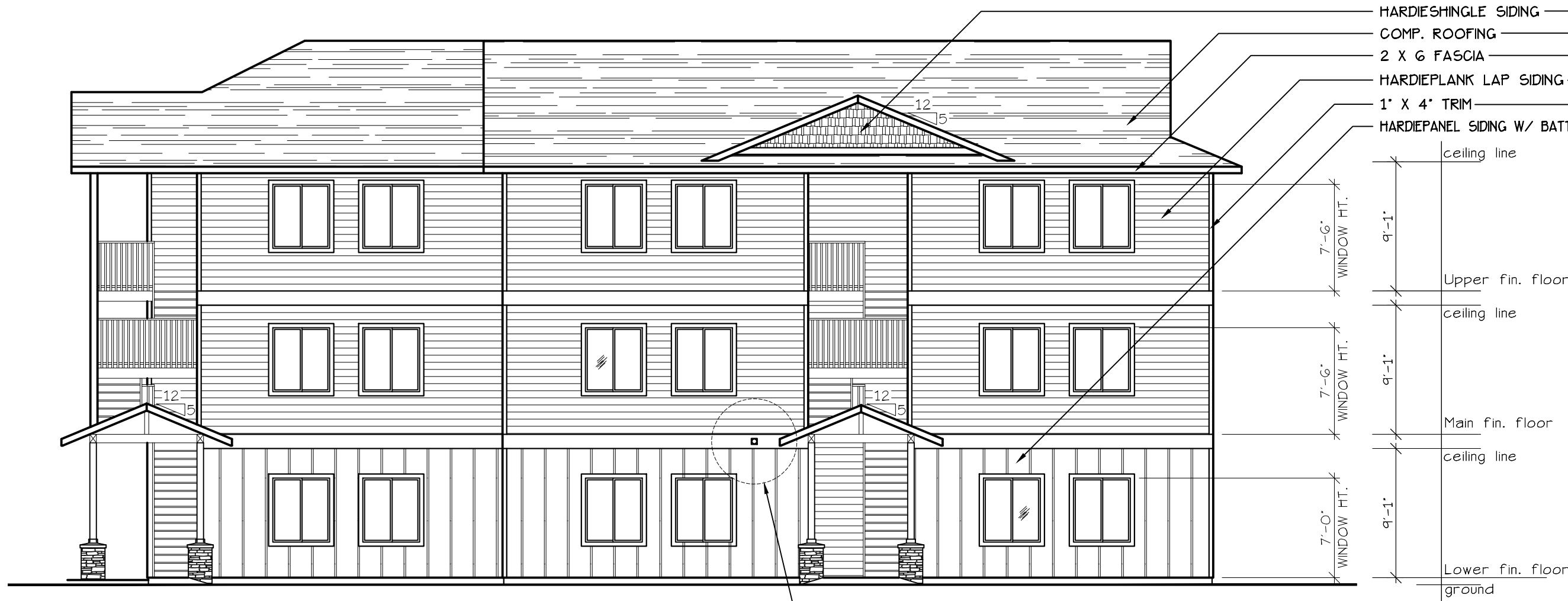
EAST ELEVATION (TYPE A UNITS) SCALE: 1/8" = 1'-0" BLD. 1
