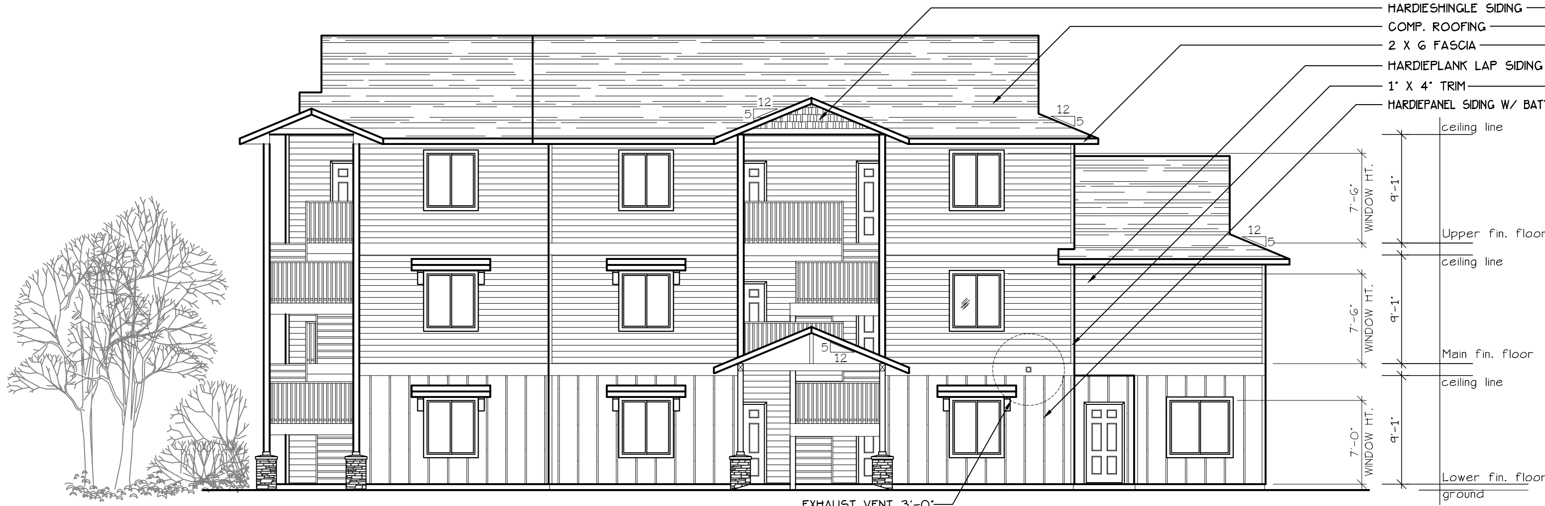
NORTH ELEVATION (TYPE C UNITS) SCALE: 1/8" = 1'-0" BLD. 2
