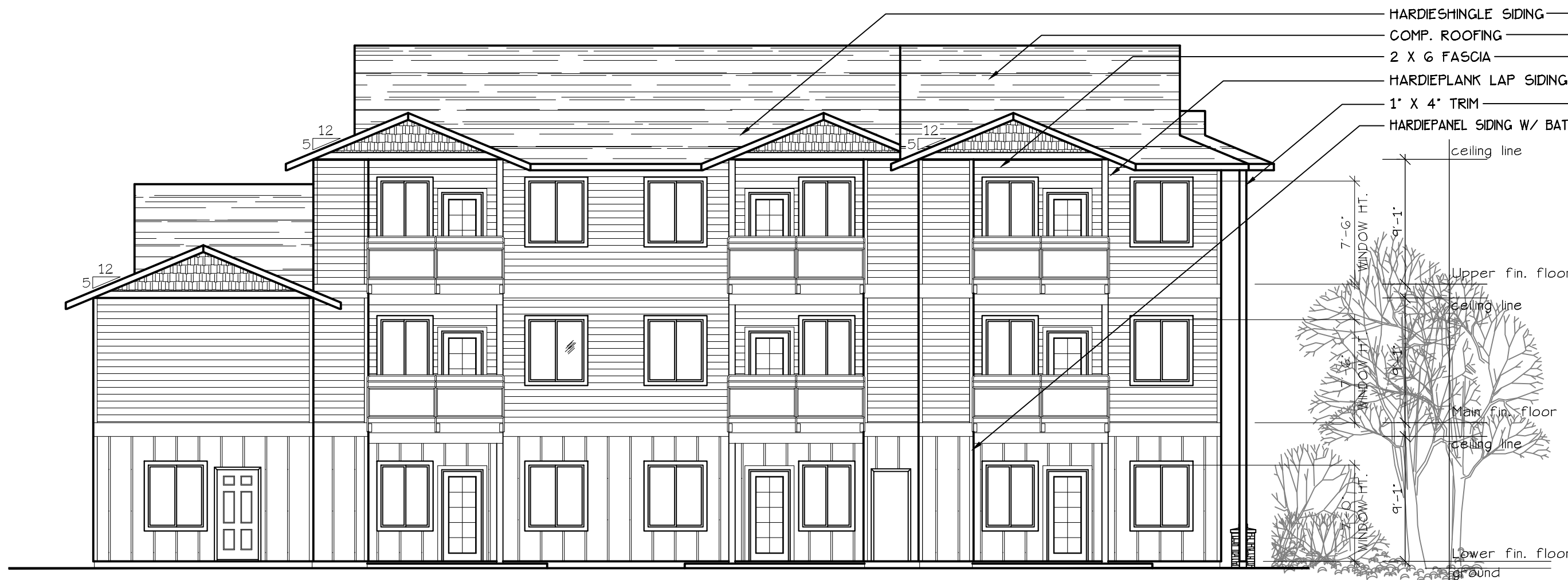
SOUTH ELEVATION (TYPE C UNITS) SCALE: 1/8" = 1'-0" BLD. 2
