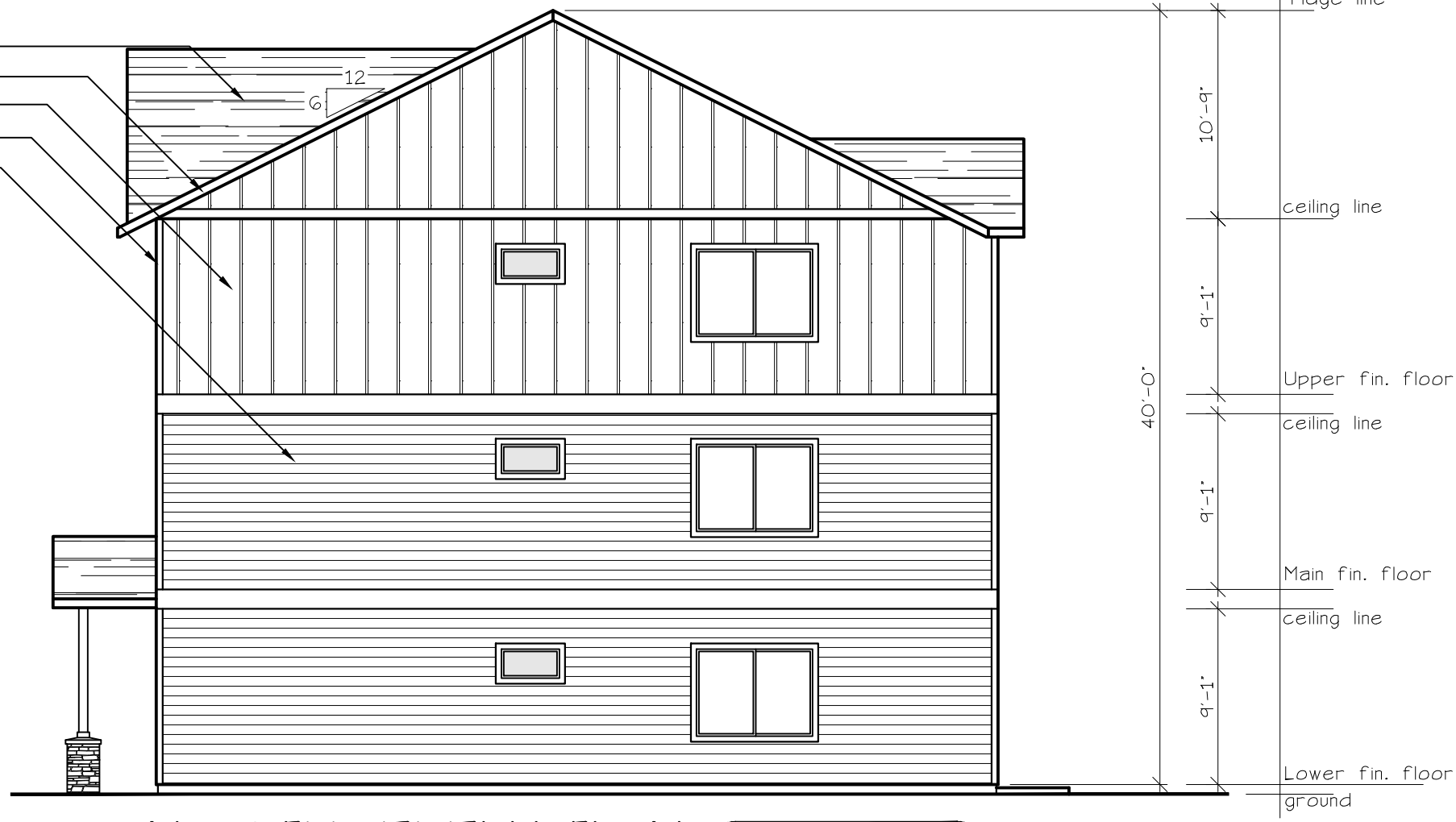
NORTH ELEVATION (TYPE A UNITS) SCALE: 1/8" = 1'-0" BLD. 4
