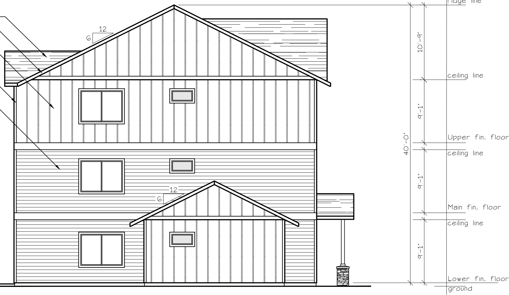
SOUTH ELEVATION (TYPE A UNITS) SCALE: 1/8" = 1'-0" BLD. 4
