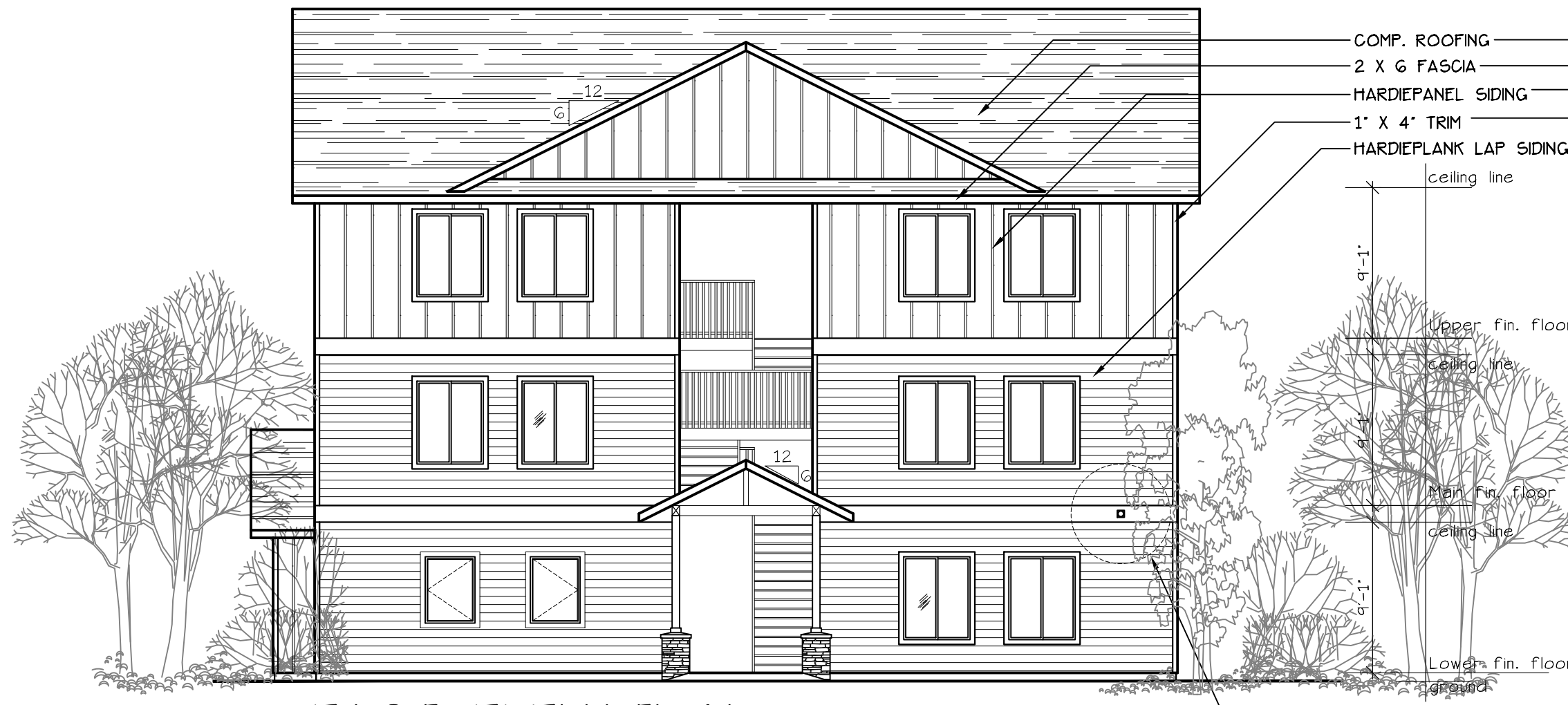
EAST ELEVATION (TYPE A UNITS) SCALE: 1/8" = 1'-0" BLD. 4
