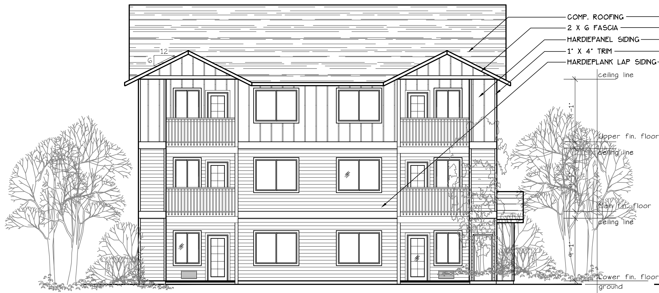
WEST ELEVATION (TYPE A UNITS) SCALE: 1/8" = 1'-0" BLD. 4
