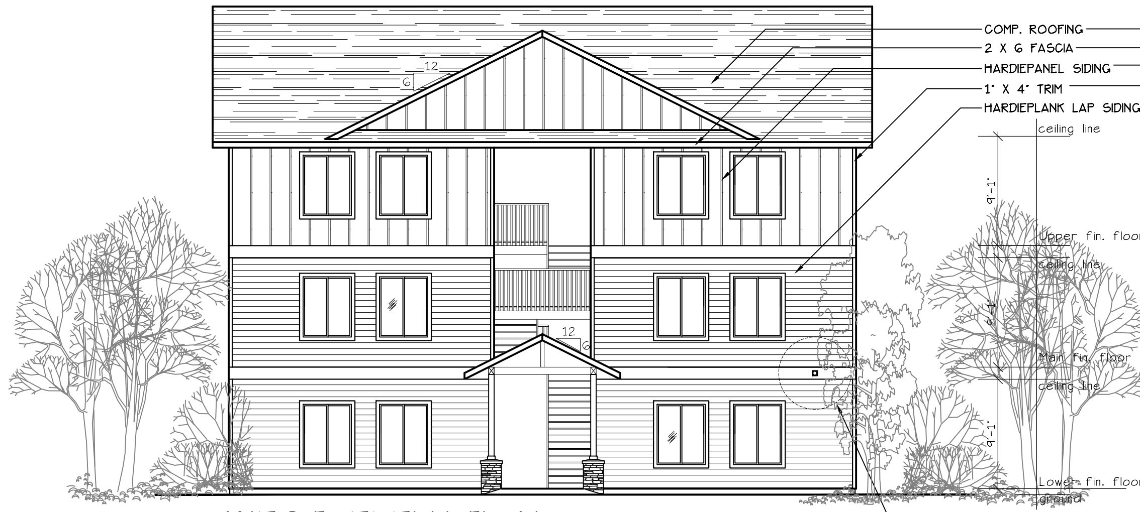
WEST ELEVATION (TYPE A UNITS) SCALE: 1/8" = 1'-0" BLD. 1
