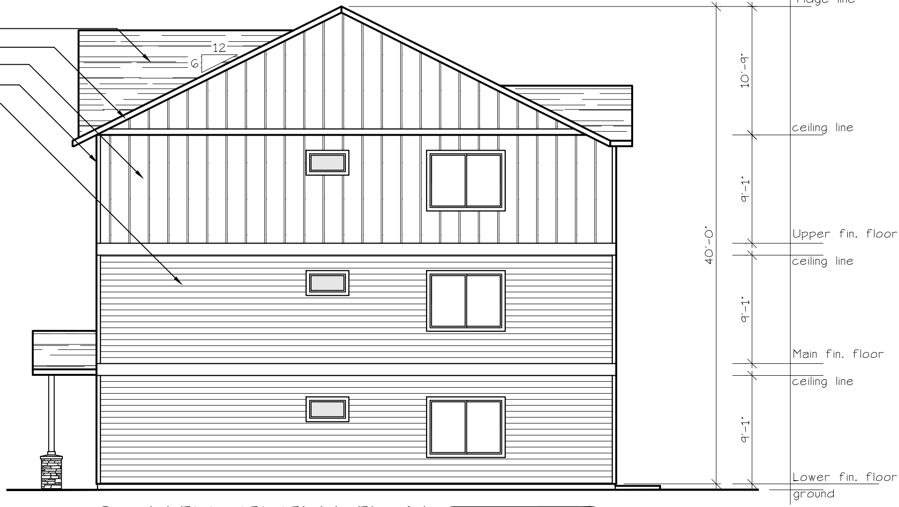
SOUTH ELEVATION (TYPE A UNITS) SCALE: 1/8" = 1'-0" BLD. 1
