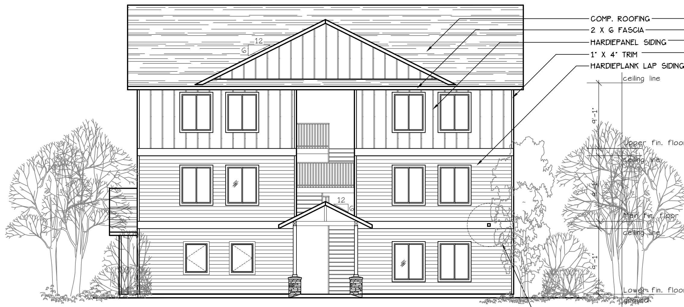
EAST ELEVATION (TYPE A UNITS) SCALE: 1/8" = 1'-0" BLD. 4
