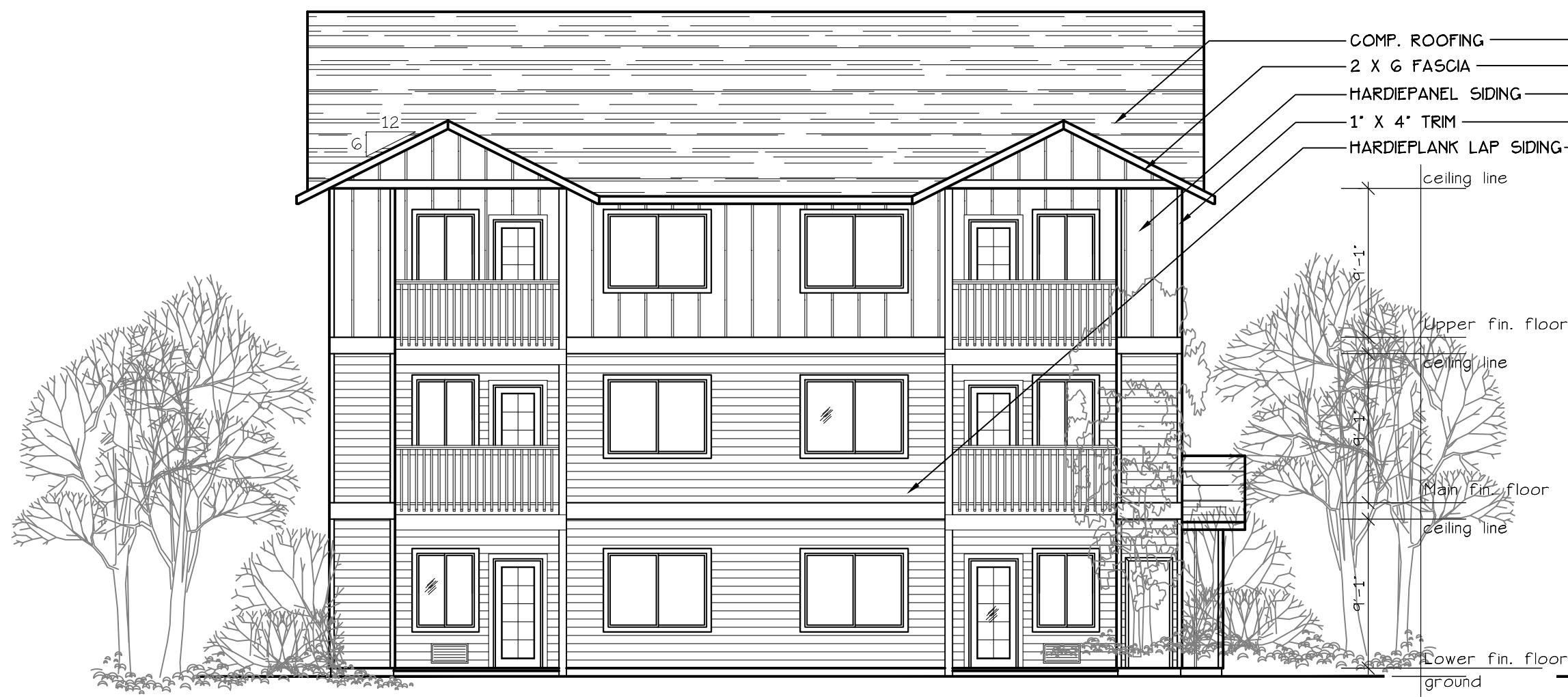
WEST ELEVATION (TYPE A UNITS) SCALE: 1/8" = 1'-0" BLD. 4
