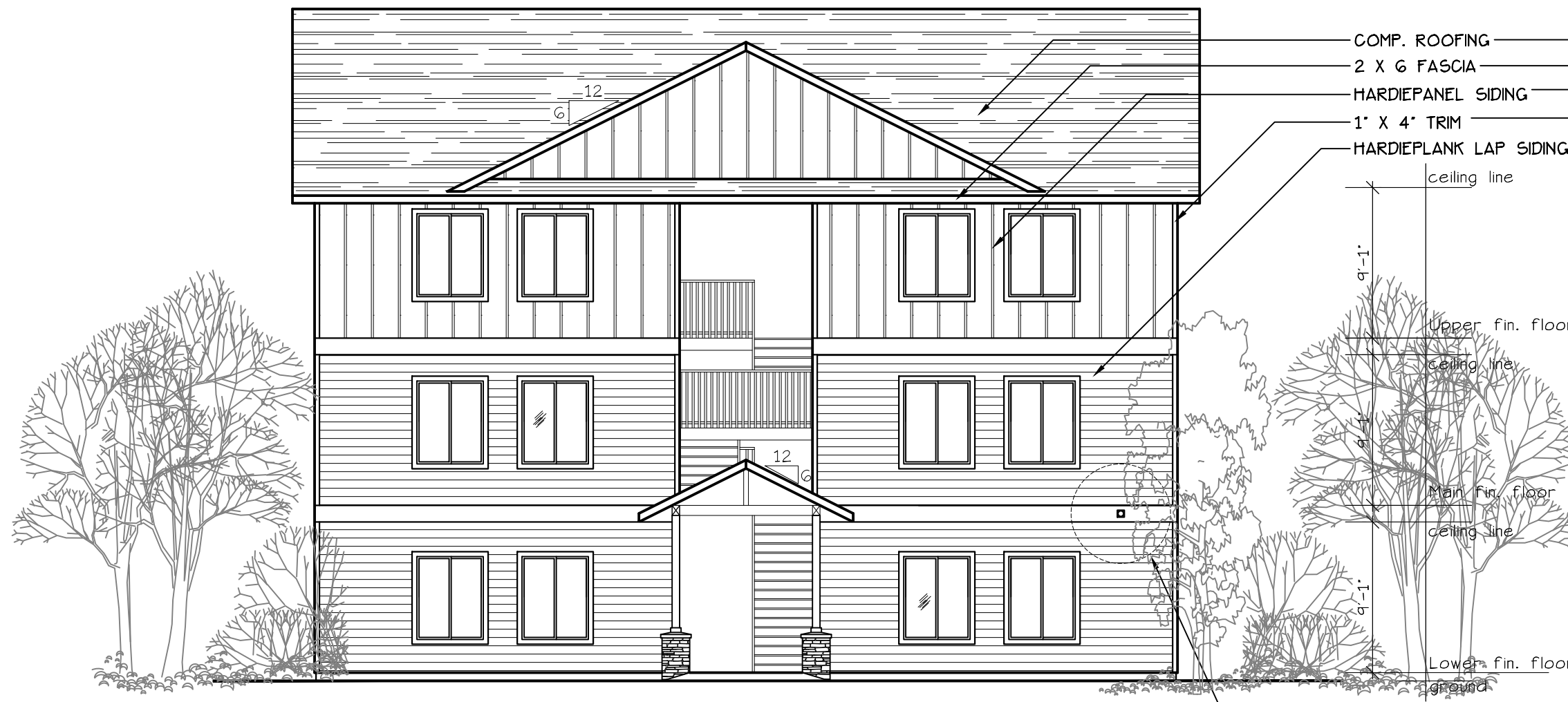
WEST ELEVATION (TYPE A UNITS) SCALE: 1/8" = 1'-0" BLD. 1
