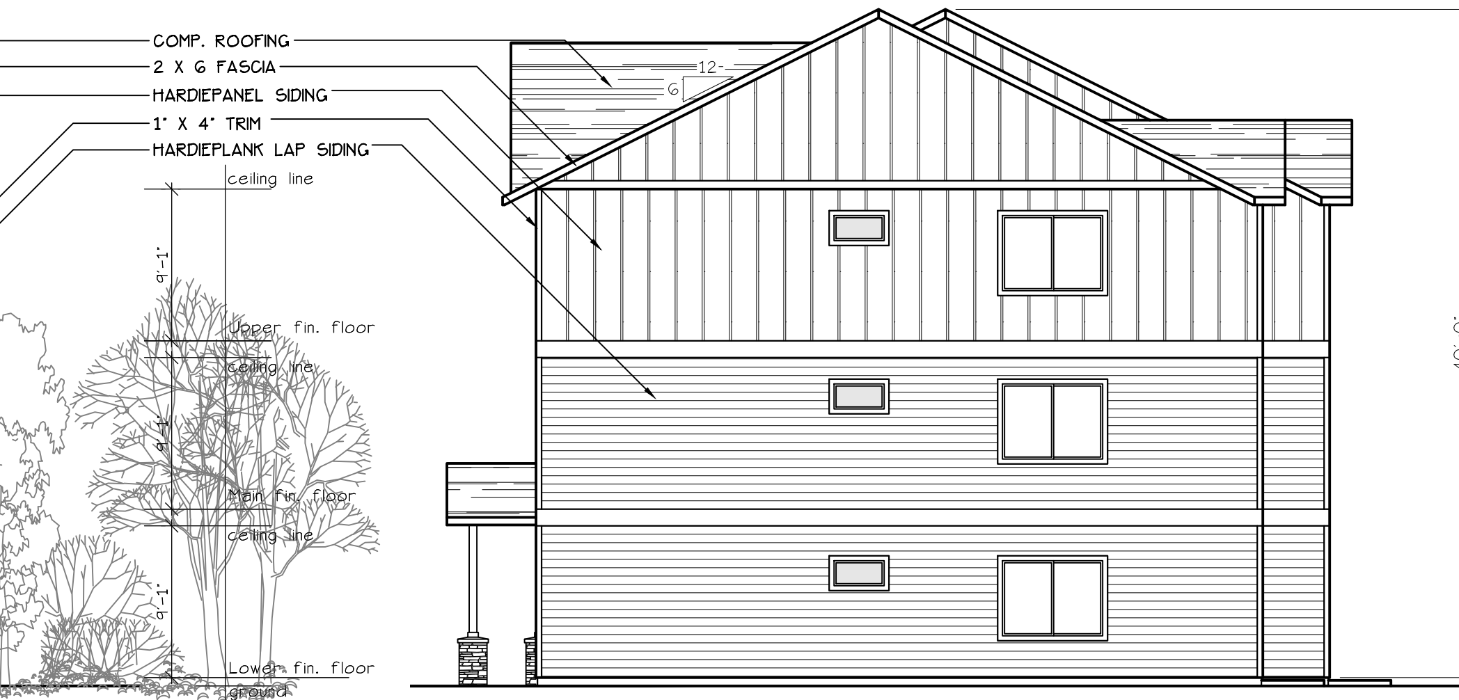
SOUTH ELEVATION (TYPE A UNITS) SCALE: 1/8" = 1'-0" BLD. 3
