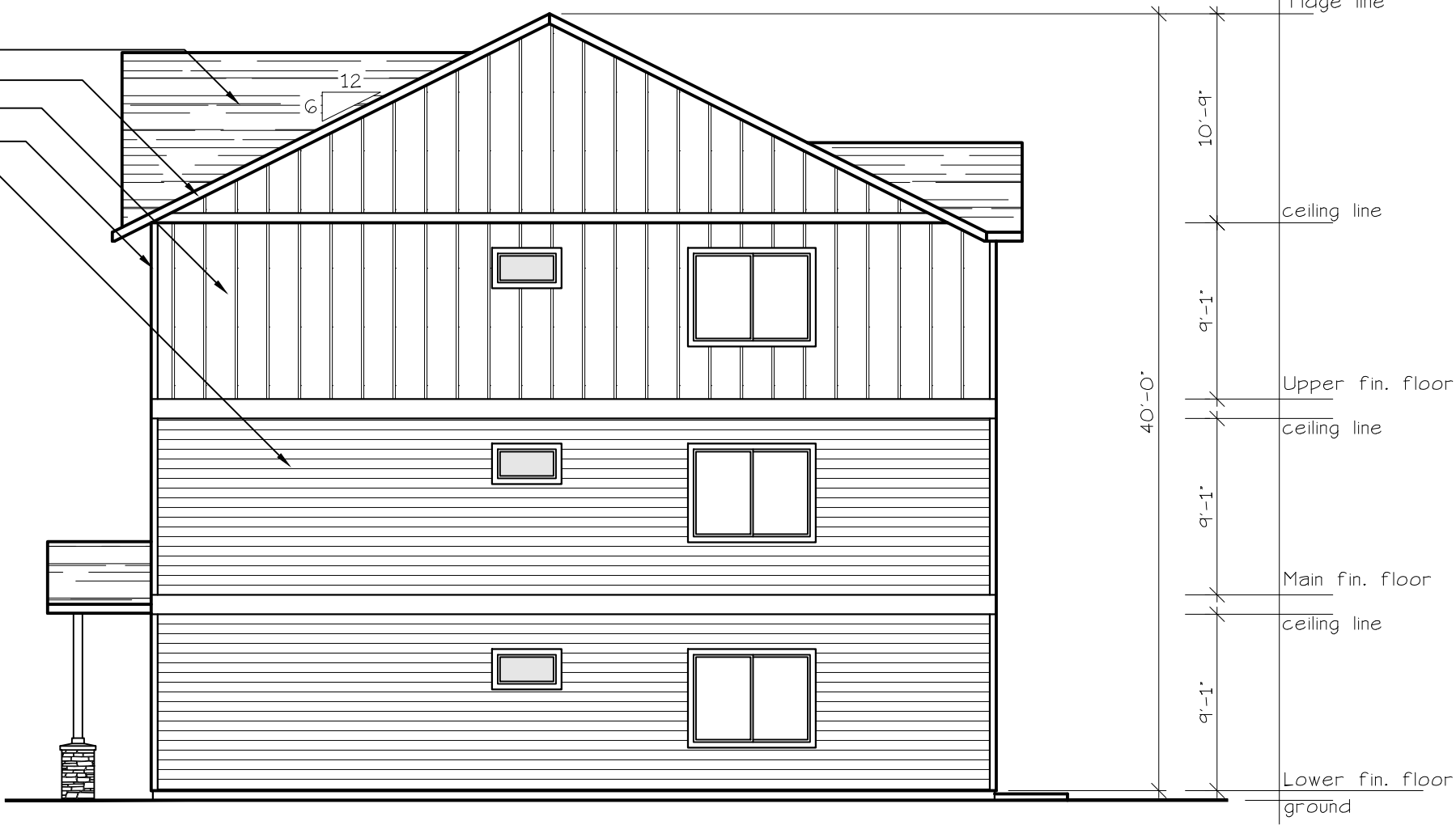
NORTH ELEVATION (TYPE A UNITS) SCALE: 1/8" = 1'-0" BLD. 4
