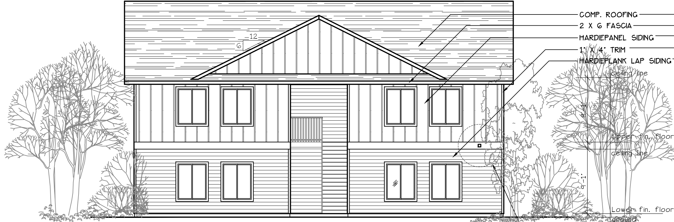
WEST ELEVATION (TYPE A UNITS) SCALE: 1/8" = 1'-0" BLD. 2
