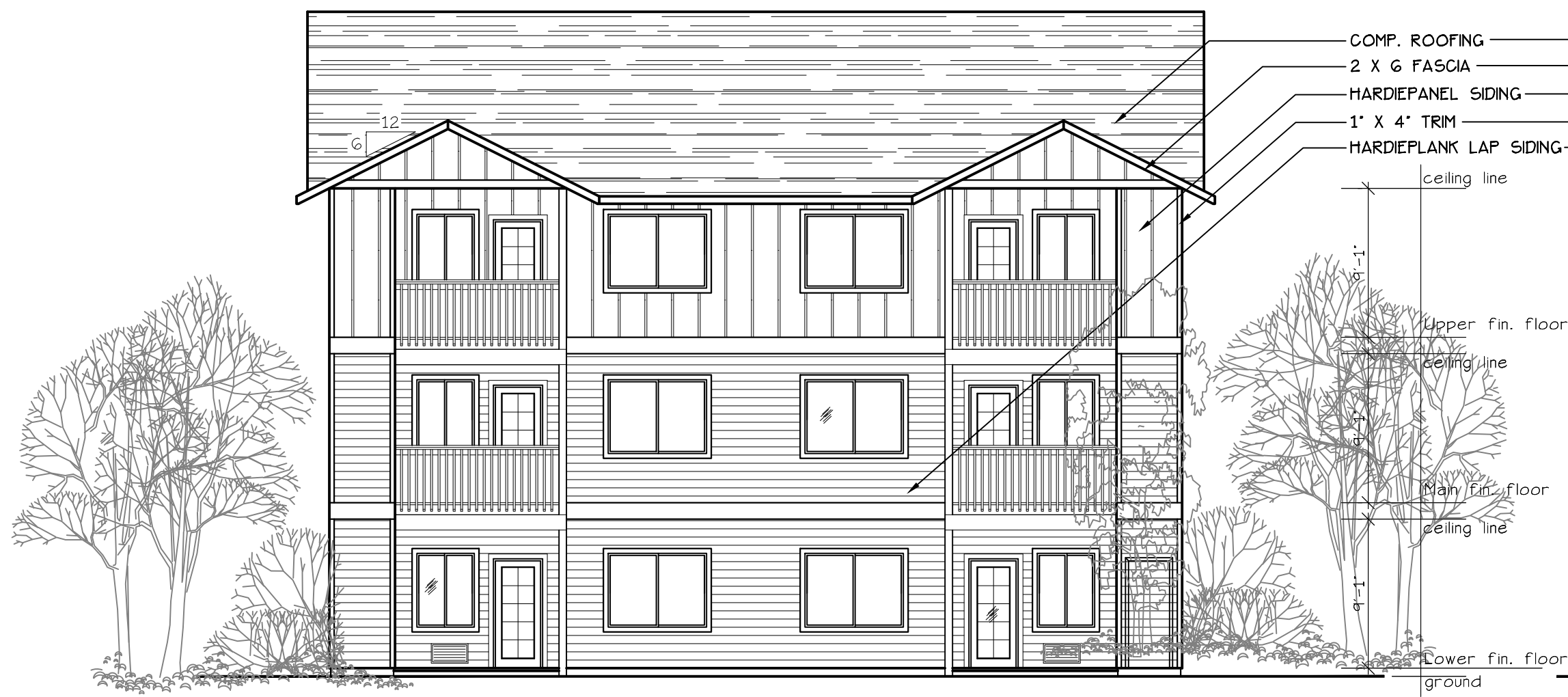
EAST ELEVATION (TYPE A UNITS) SCALE: 1/8" = 1'-0" BLD. 1
