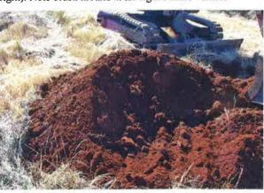
Decomposed Sentinel Bluff basalt spoils from test pit TP-1
