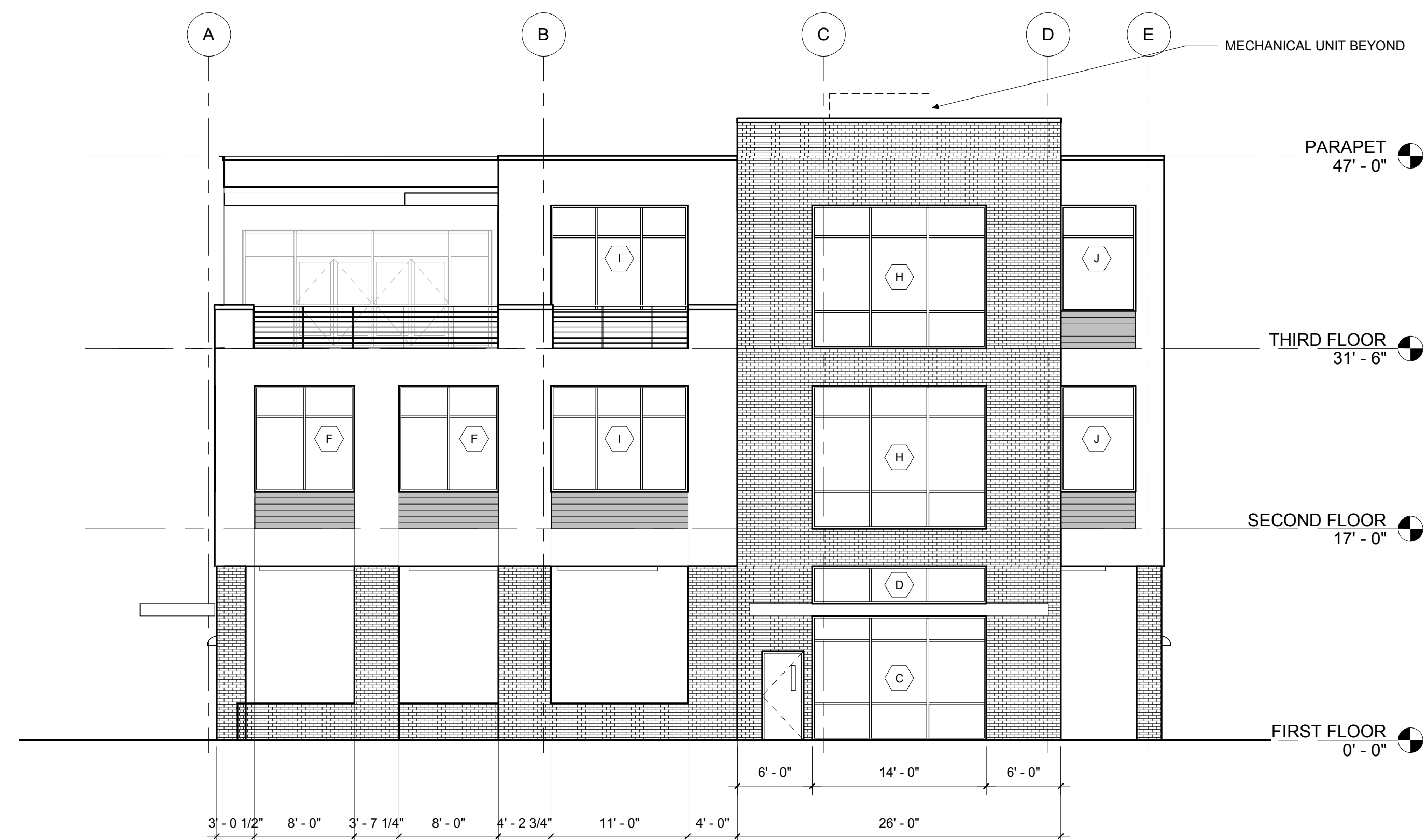
Architectural drawing of the West Elevation of a building. The drawing shows the First, Second, and Third floors, along with a Parapet. The building is divided into 11 vertical sections, numbered 1 through 11. The First Floor is 0' - 0" high, the Second Floor is 17' - 0" high, and the Third Floor is 31' - 6" high. The Parapet is 47' - 0" high. The drawing includes a scale bar (1/8" = 1'-0") and a north arrow. The building features a central entrance on the First Floor, a large glass facade on the Second Floor, and a series of windows on the Third Floor. A "maps" logo is visible on the Second Floor facade.
