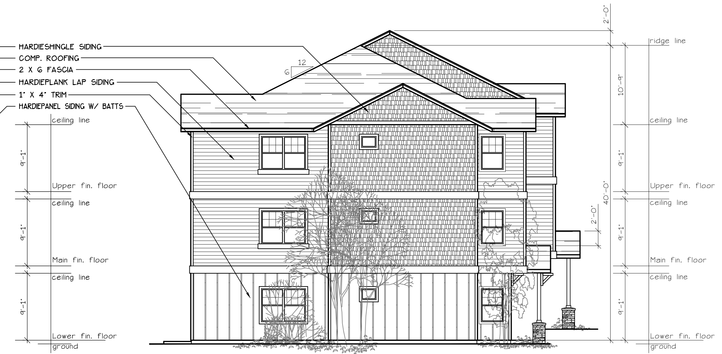
NORTH ELEVATION (TYPE A UNITS) SCALE: 1/8" = 1'-0" BLD. 17
