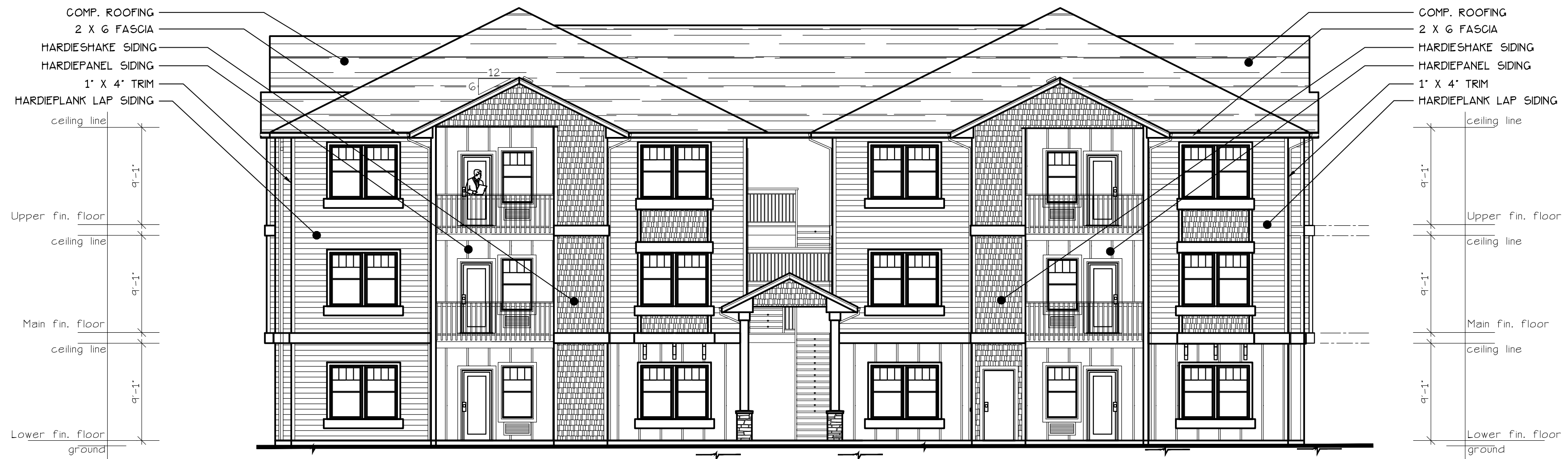
REAR ELEVATION (BLD. 2.14) SCALE: 1/8" = 1'-0" TYPE E UNIT
