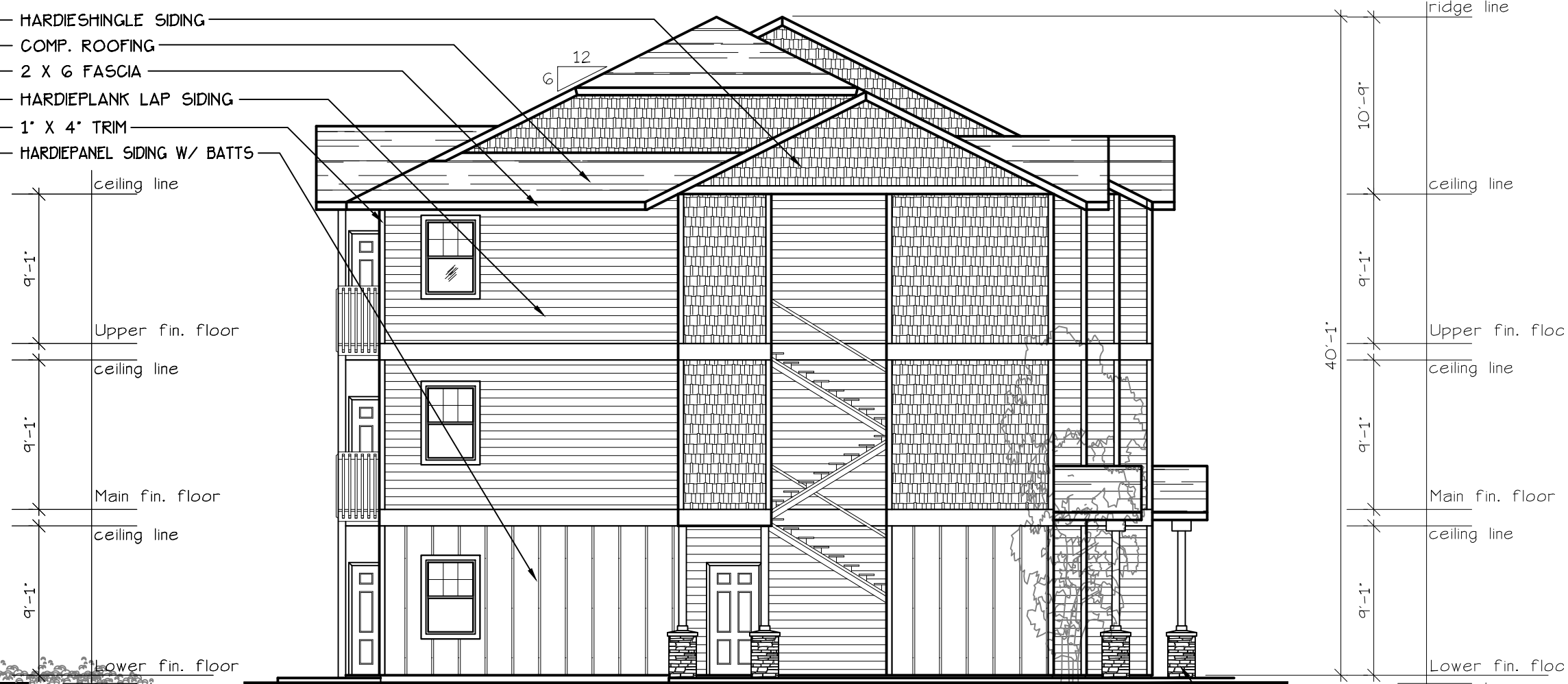
WEST ELEVATION (TYPE A UNITS) SCALE: 1/8" = 1'-0" BLD. 12
