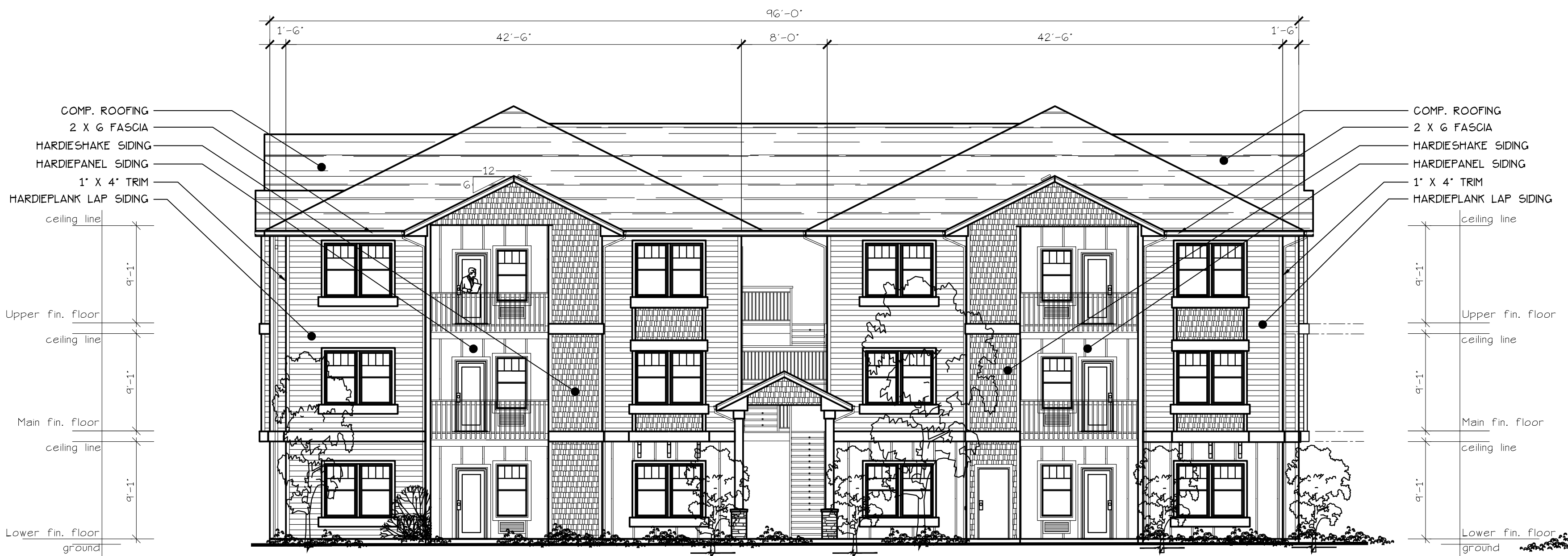
FRONT ELEVATION (BLD. 2.14) SCALE: 1/8" = 1'-0" TYPE E UNIT
