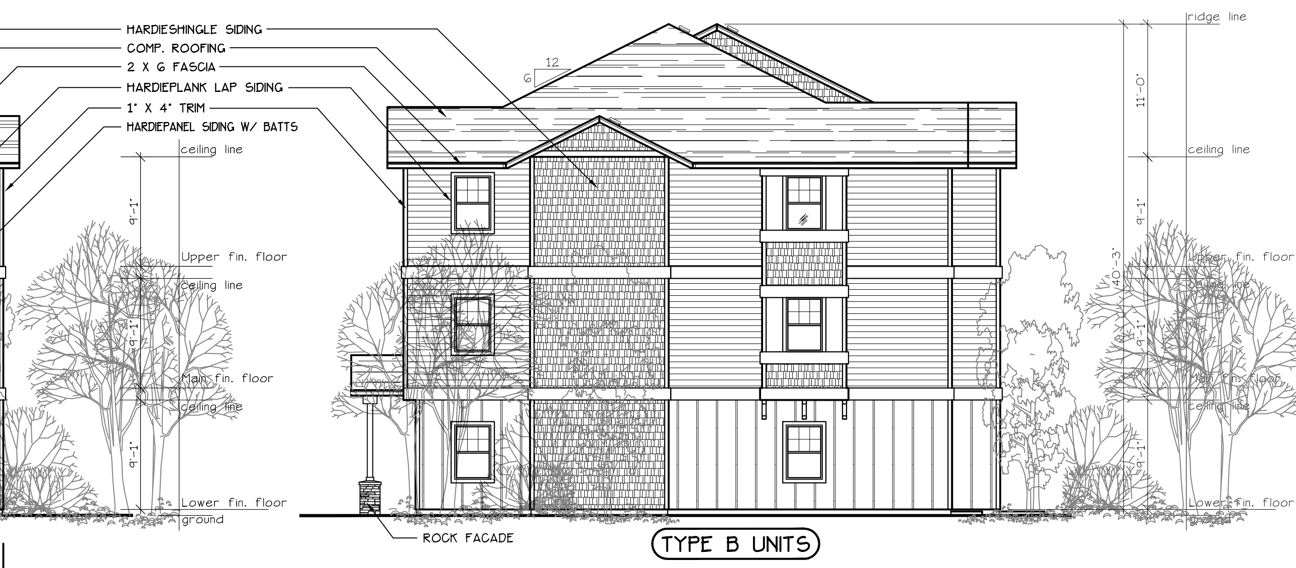
TYPE B UNITS NORTH ELEVATION (BLD. 3) SCALE: 1/8" = 1'-0"
