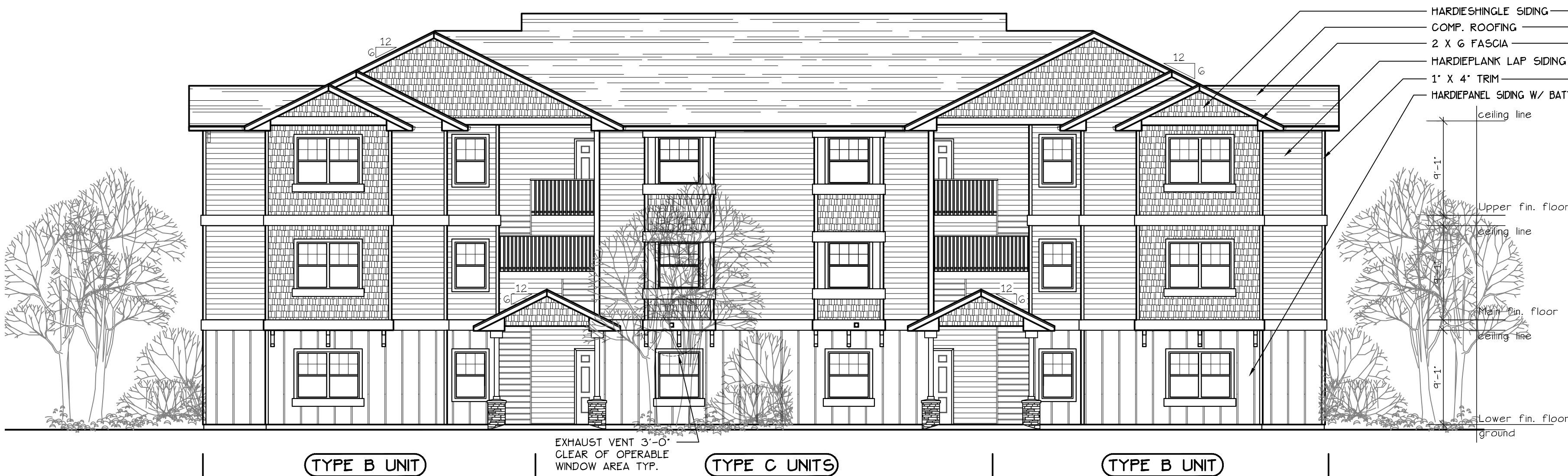
FRONT ELEVATION (BLD. 8-11.15) SCALE: 1/8" = 1'-0"
