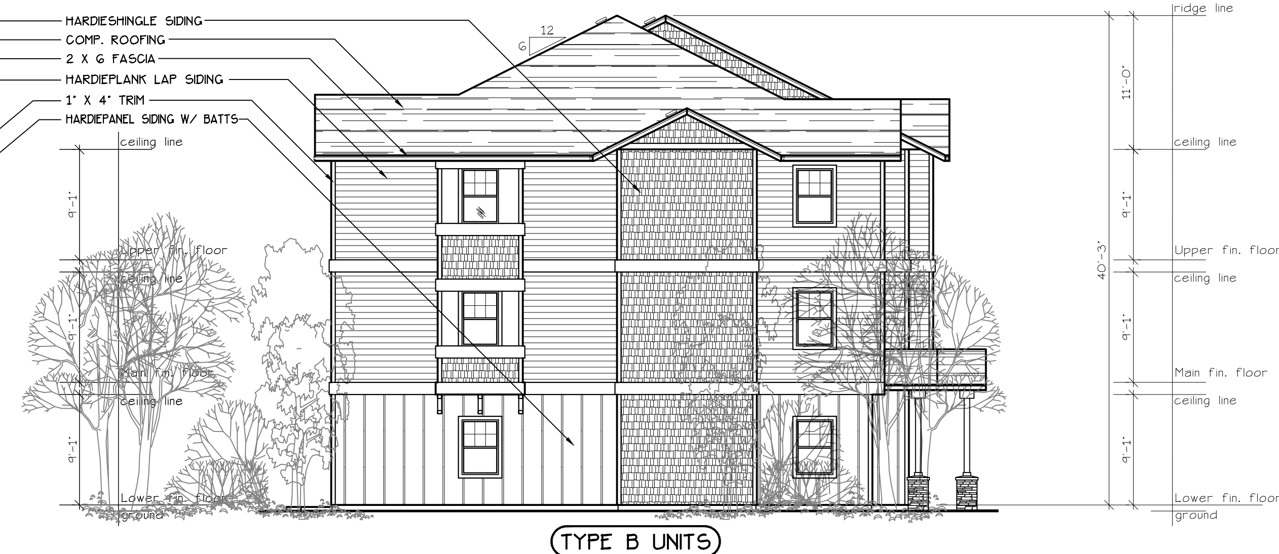
TYPE B UNITS NORTH ELEVATION (BLD. 3) SCALE: 1/8" = 1'-0"
