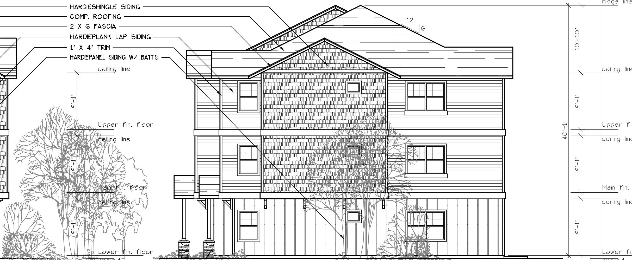
EAST ELEVATION (TYPE A UNITS) SCALE: 1/8" = 1'-0" BLD. 12
