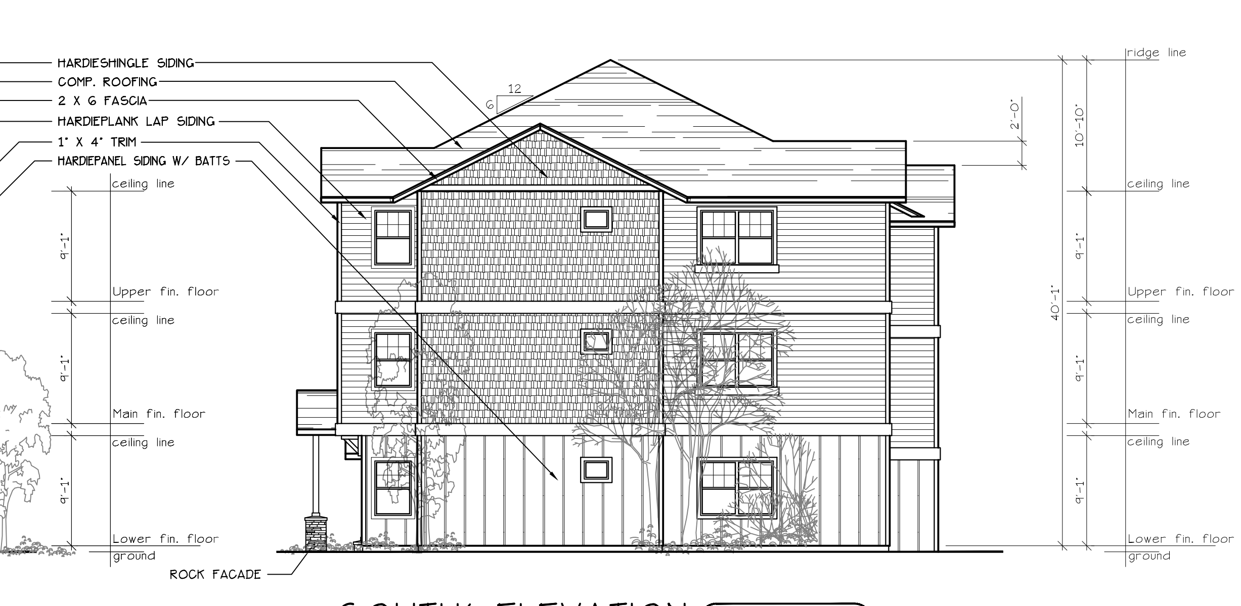
SOUTH' ELEVATION (TYPE A UNITS) SCALE: 1/8" = 1'-0" BLD. 17
