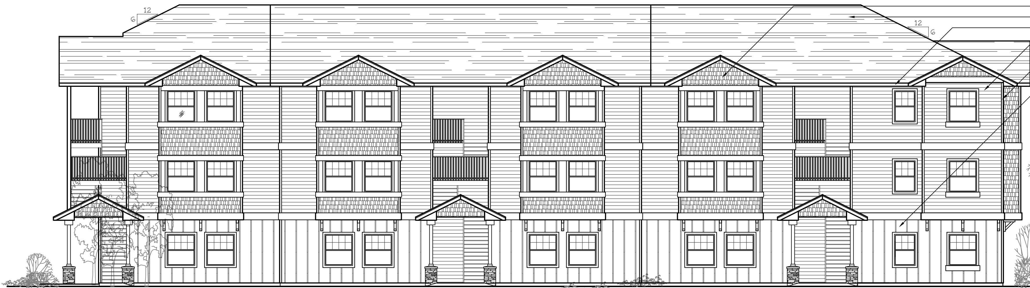
SOUTH ELEVATION (TYPE A UNITS) SCALE: 1/8" = 1'-0" BLD. 12
