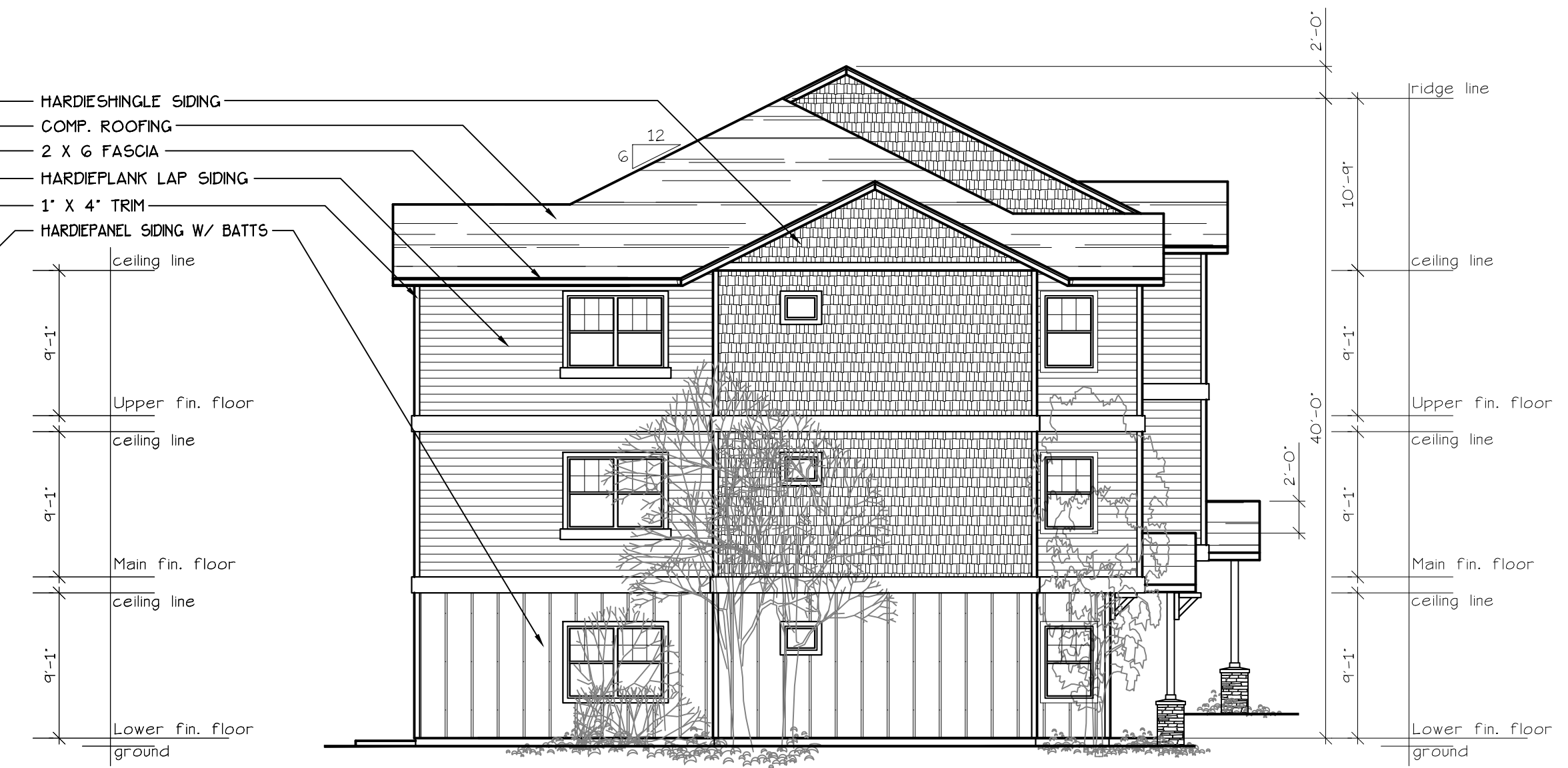
NORTH ELEVATION (TYPE A UNITS) SCALE: 1/8" = 1'-0" BLD. 17
