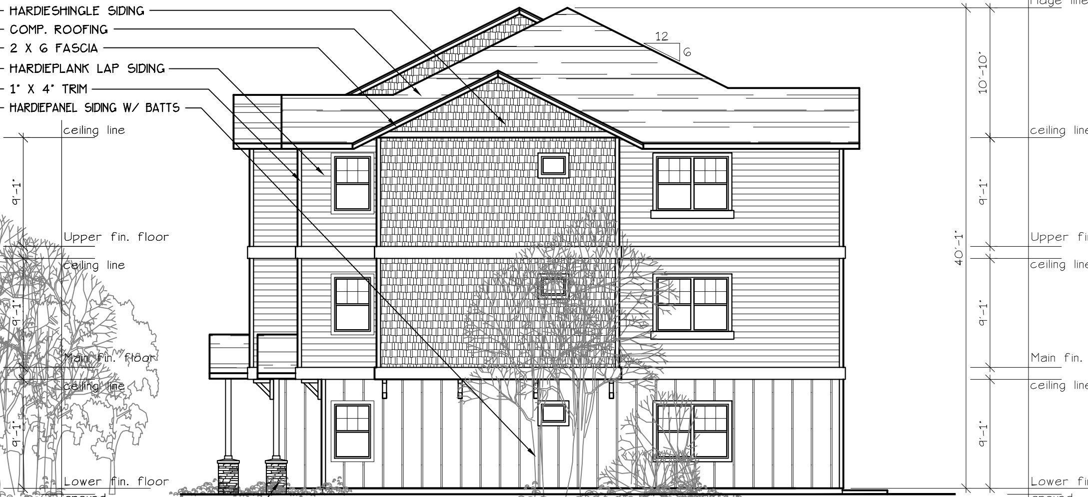
EAST ELEVATION (TYPE A UNITS) SCALE: 1/8" = 1'-0" BLD. 12
