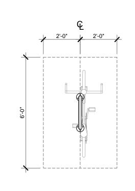
**BIKE RACK PLAN DETAIL** SCALE: 3/4" = 1'-0"
