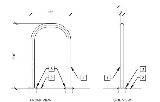
1 2" DIA. SCHEDULE 40 PIPE WITH EMBEDDED ANCHOR MOUNT, POWDER COAT FINISH
