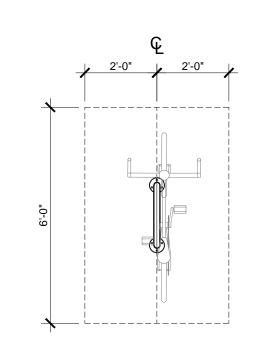
**BIKE RACK PLAN DETAIL** SCALE: 3/4" = 1'-0"
