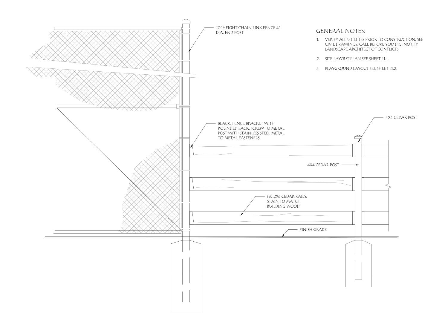
CHAIN LINK TO WOOD RAIL FENCE DETAIL
