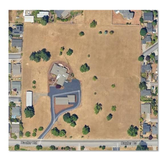
As a part of further development, Snowball Avenue (on the east) will need to be connected to the new Snowline Street out to Baxter. The elevation of the existing Snowball Avenue is 468.89. This street needs to intersect with Snowline which has an elevation of approximately 488 at the intersection with Baxter and 498.28 to the north.
