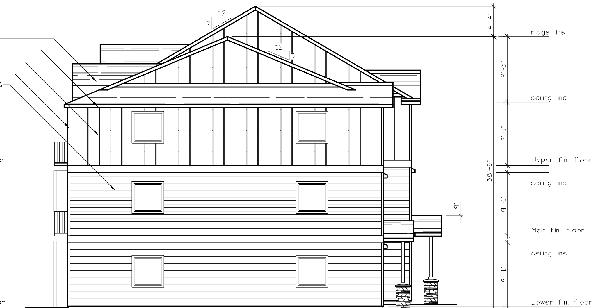
SOUTH ELEVATION (TYPE B UNITS) SCALE: 1/8" = 1'-0" BLD. 10
