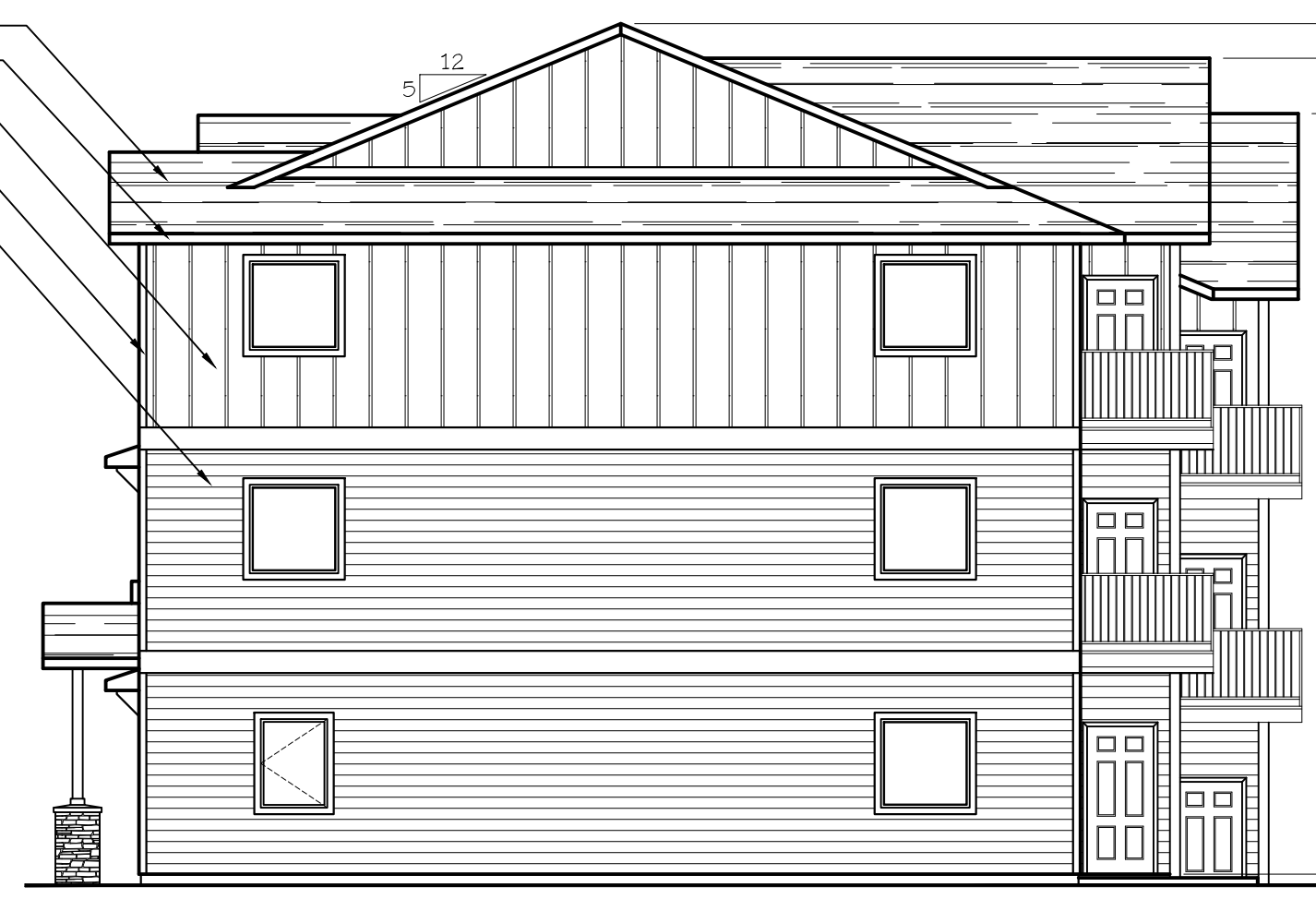
WEST ELEVATION (TYPE C UNITS) SCALE: 1/8" = 1'-0" BLD. 2
