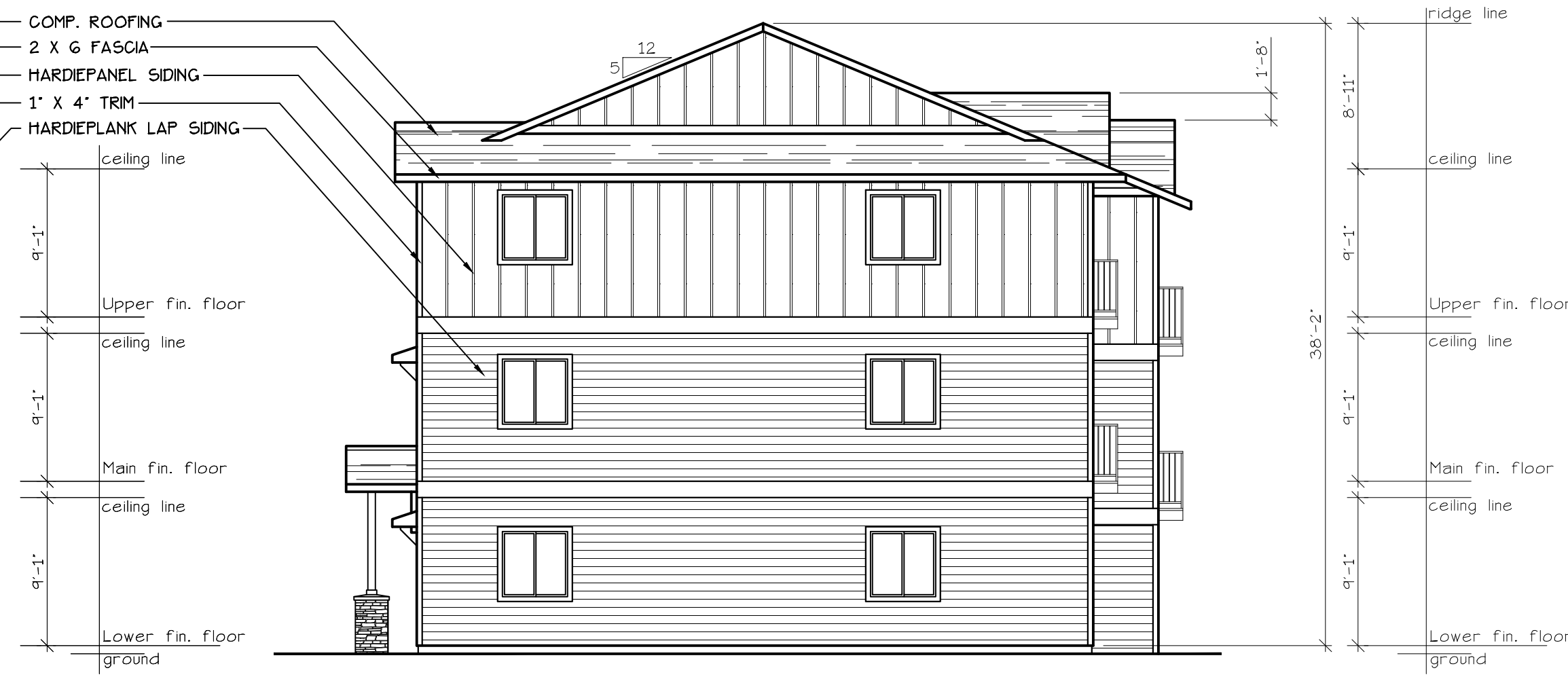
WEST ELEVATION (TYPE A UNITS) SCALE: 1/8" = 1'-0" BLD. 3
