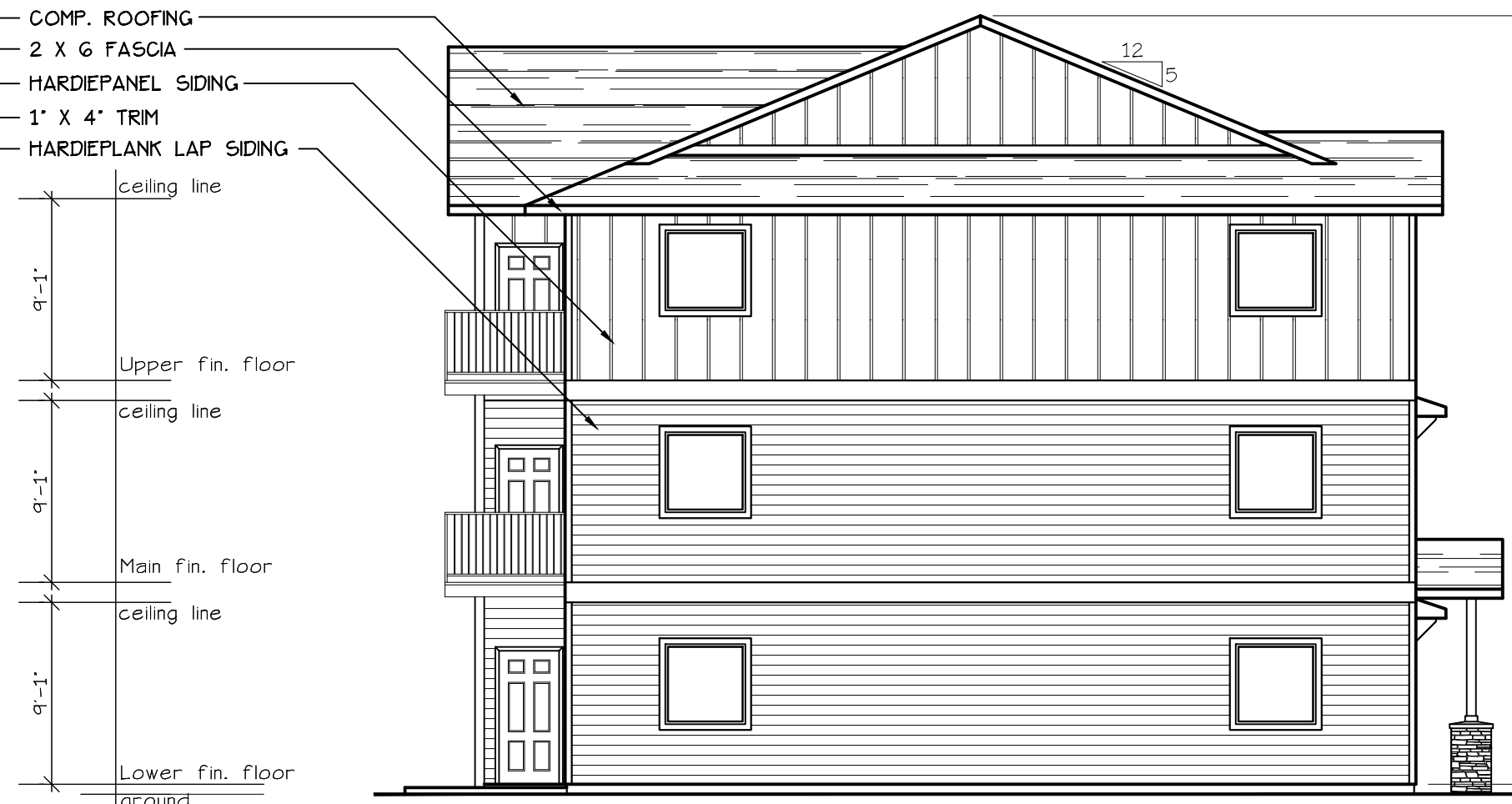
EAST ELEVATION (TYPE C UNITS) SCALE: 1/8" = 1'-0" BLD. 5
