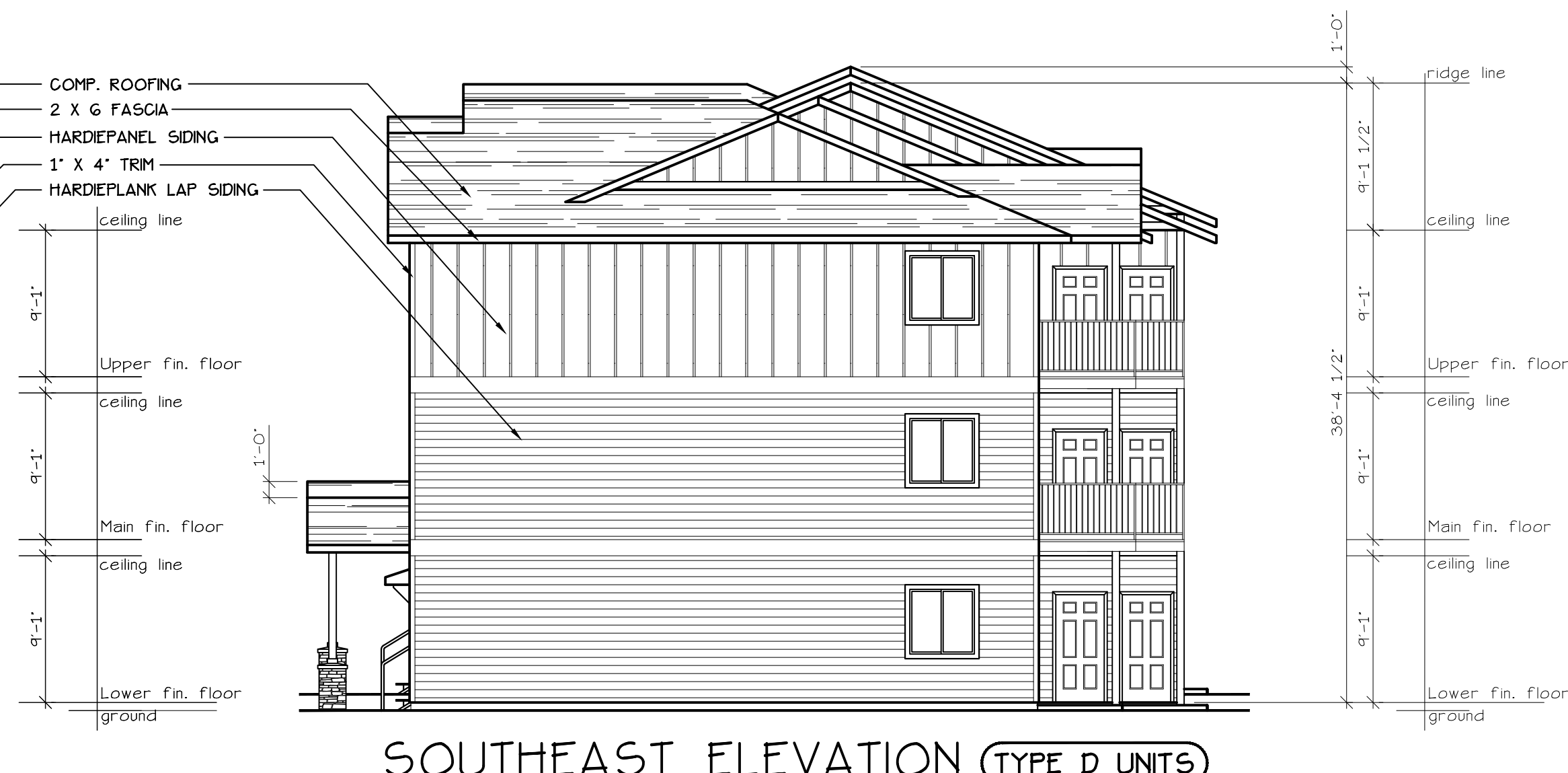
SOUTHEAST ELEVATION (TYPE D UNITS) SCALE: 1/8" = 1'-0" (BLD. 6)
