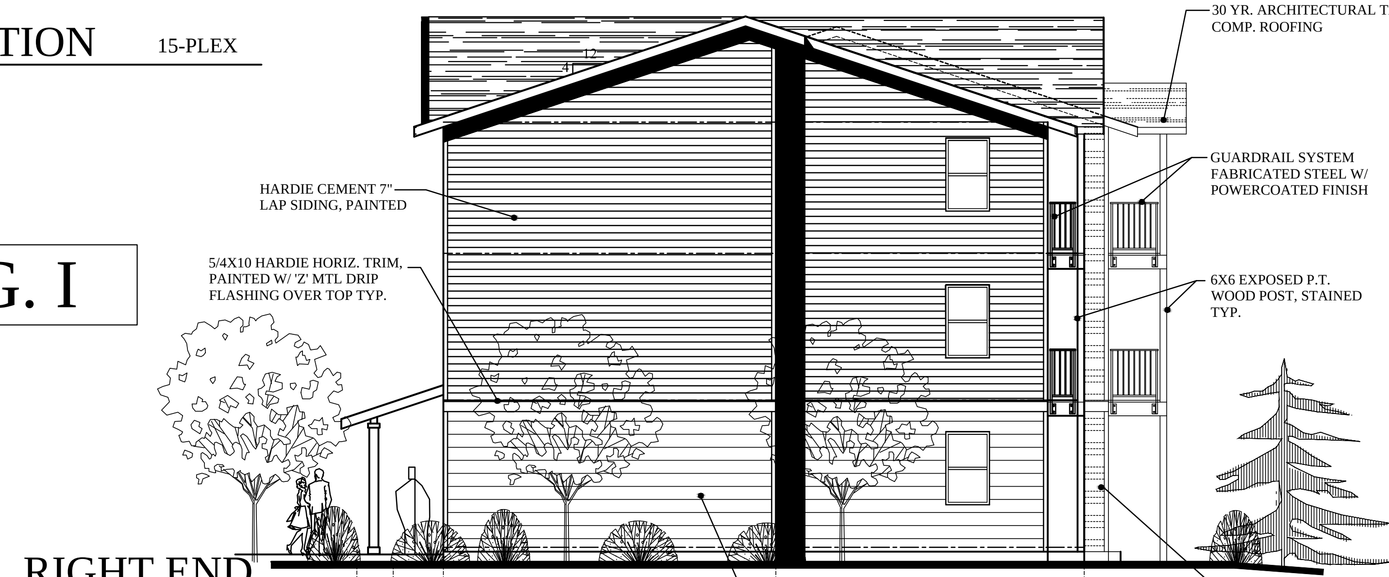
RIGHT END ELEVATION 15-PLEX
