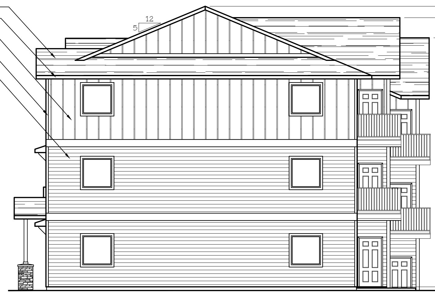
WEST ELEVATION (TYPE C UNITS) SCALE: 1/8" = 1'-0" BLD. 4
