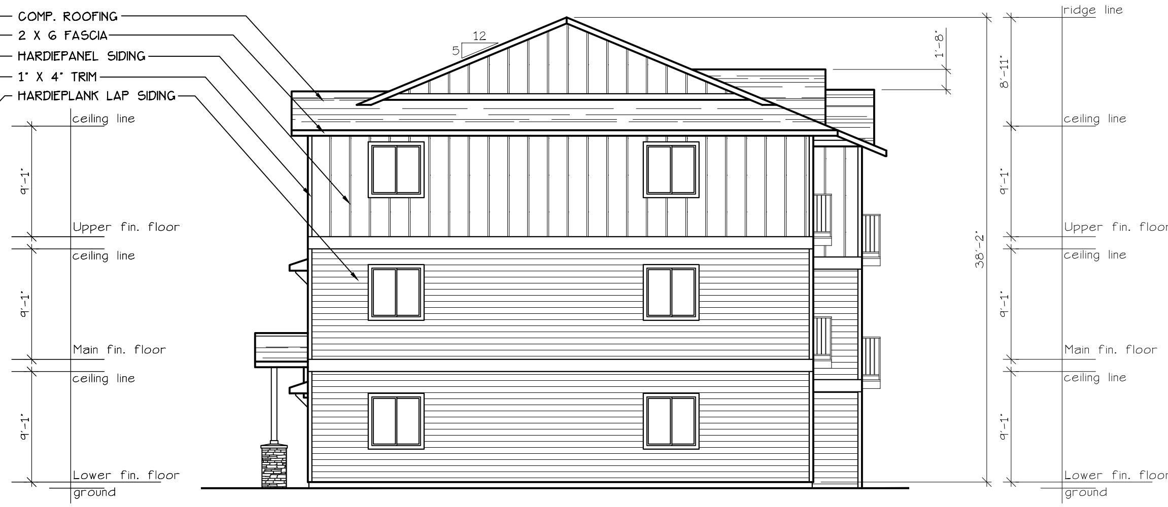
WEST ELEVATION (TYPE A UNITS) SCALE: 1/8" = 1'-0" BLD. 3
