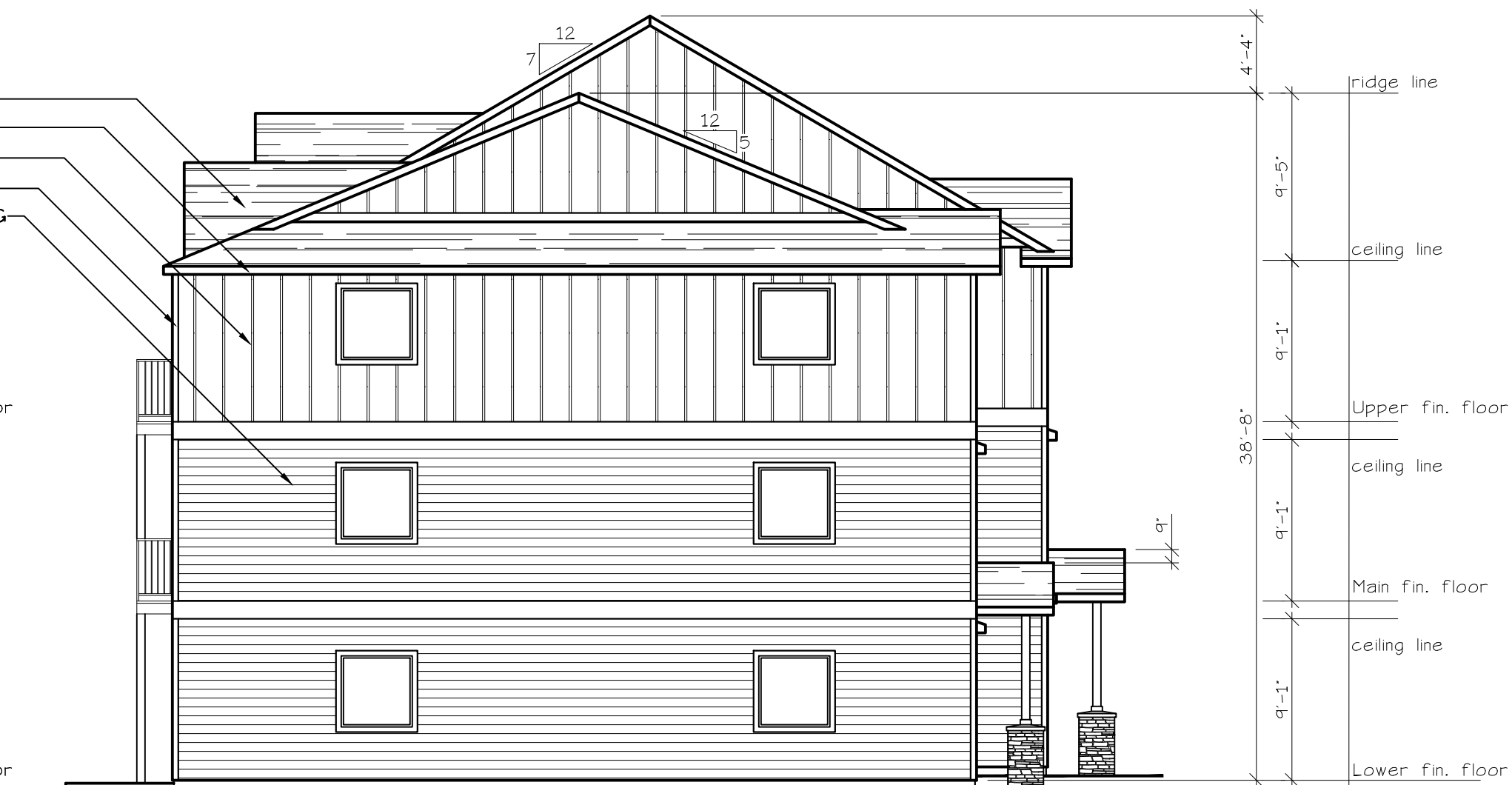
SOUTH ELEVATION (TYPE B UNITS) SCALE: 1/8" = 1'-0" BLD. 10
