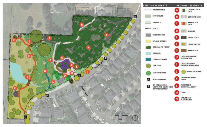
Pictured above is a graphic featuring the second concept for Bailey Ridge Park. Proposed elements are identified on the graphic and in the legend with a red circle that contains a white letter.
