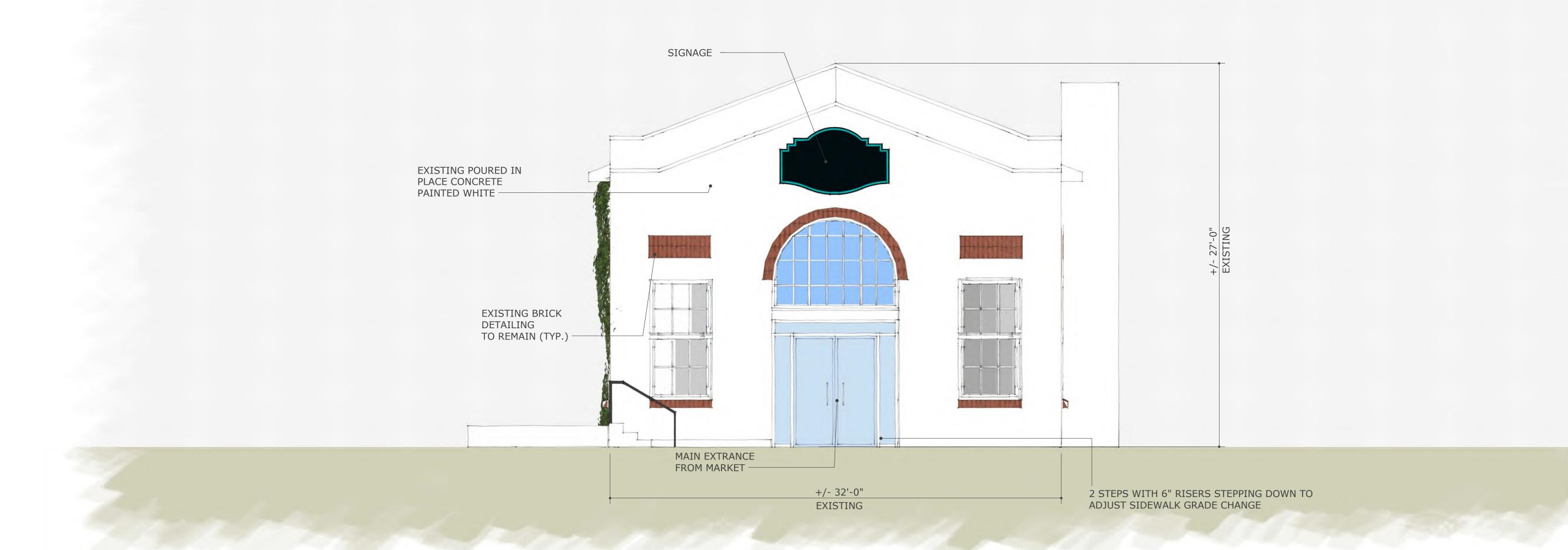
NOTE: CURRENTLY, THIS FACADE IS COVERED BY A PREVIOUS ADDITION, WHICH IS TO BE DEMOLISHED. ALTERED PORTION OF FACADE IS LESS THAN 10% OF THE OVERALL FACADE.
