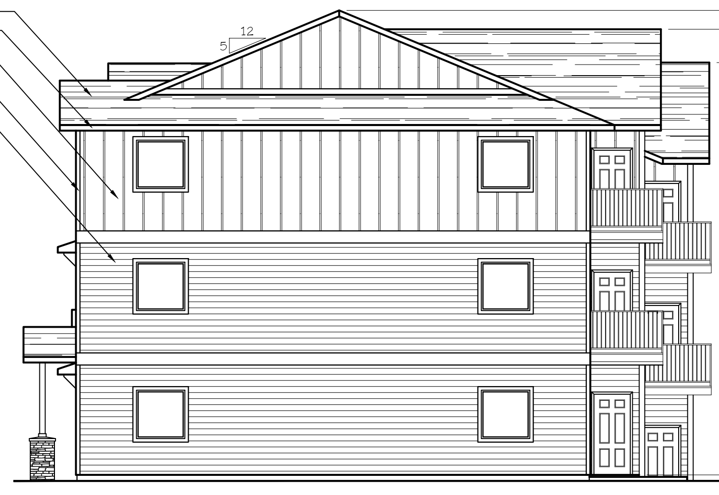
WEST ELEVATION (TYPE C UNITS) SCALE: 1/8" = 1'-0" BLD. 4
