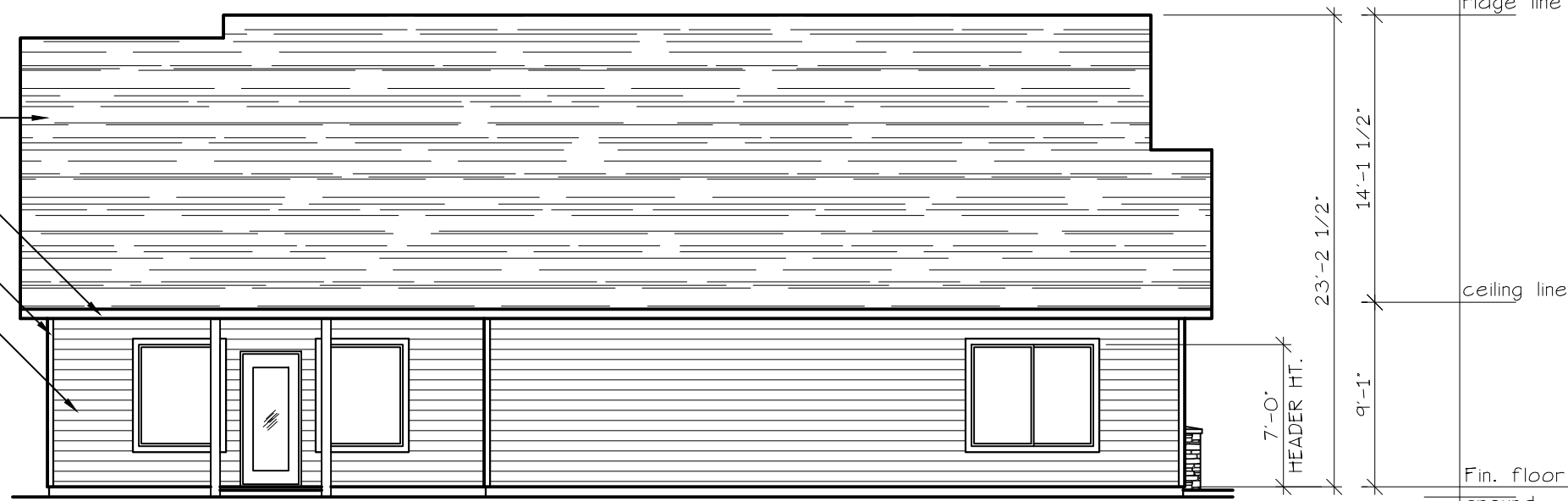
WEST ELEVATION (RECREATION BLD.) SCALE: 1/8" = 1'-0" BLD. 12
