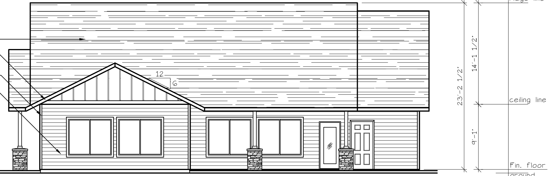
EAST ELEVATION (RECREATION BLD.) SCALE: 1/8" = 1'-0" BLD. 12
