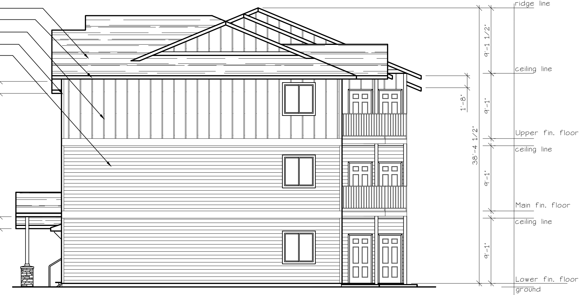
WEST ELEVATION (TYPE D UNITS) SCALE: 1/8" = 1'-0" (BLD. 12)
