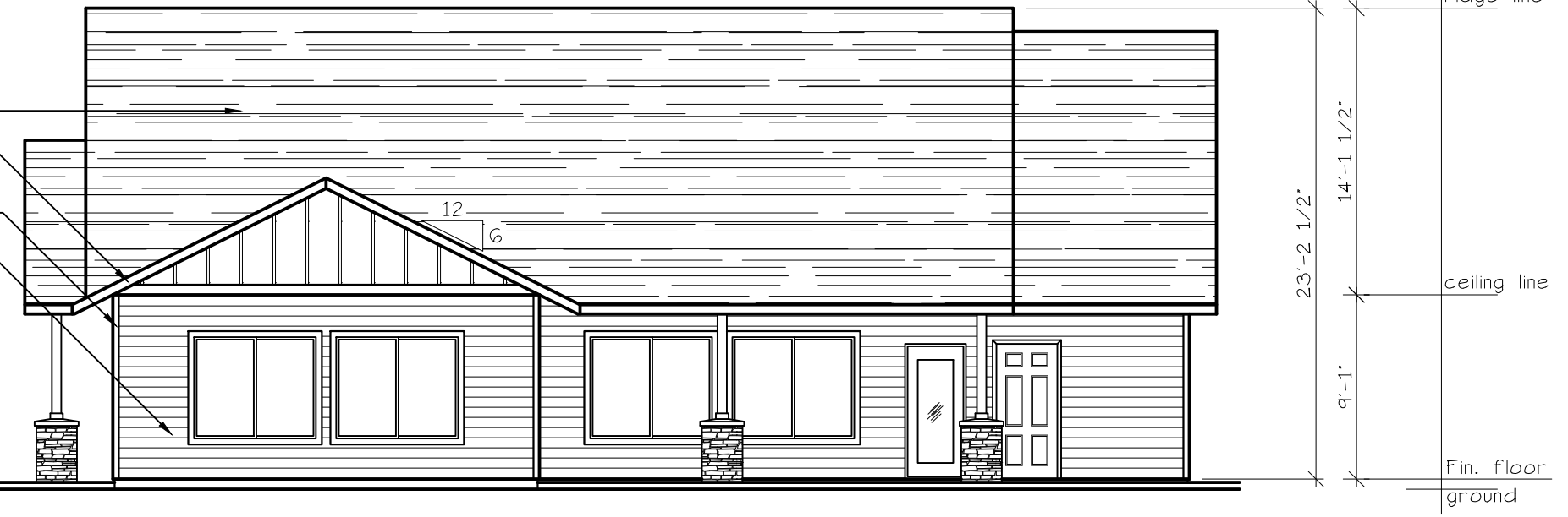
EAST ELEVATION (RECREATION BLD.) SCALE: 1/8" = 1'-0" BLD. 11
