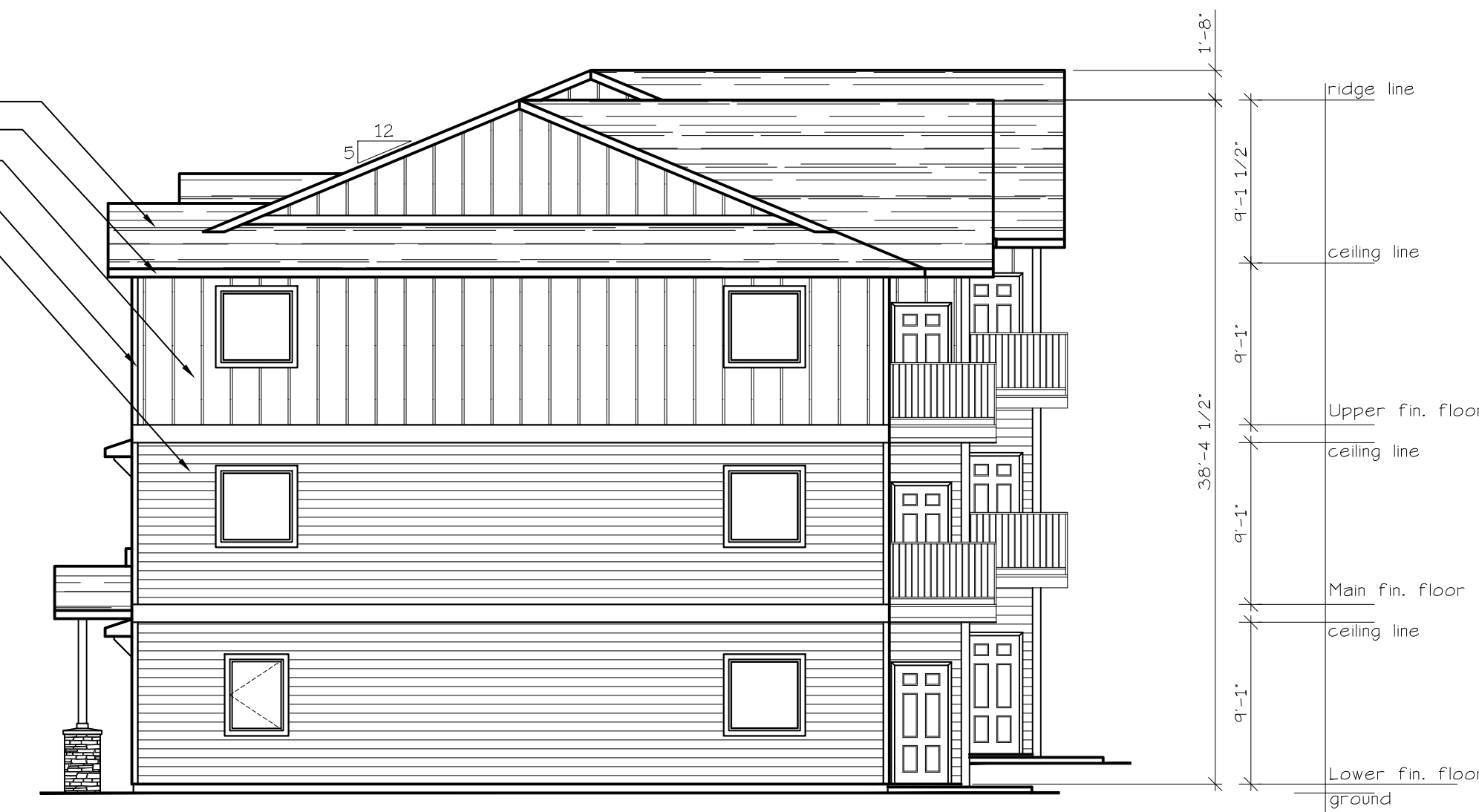
EAST ELEVATION (TYPE C UNITS) SCALE: 1/8" = 1'-0" (BLD. 9)
