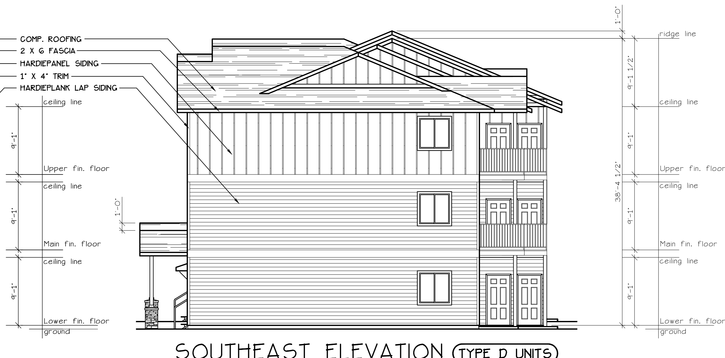
SOUTHEAST ELEVATION (TYPE D UNITS) SCALE: 1/8" = 1'-0" (BLD. 6)
