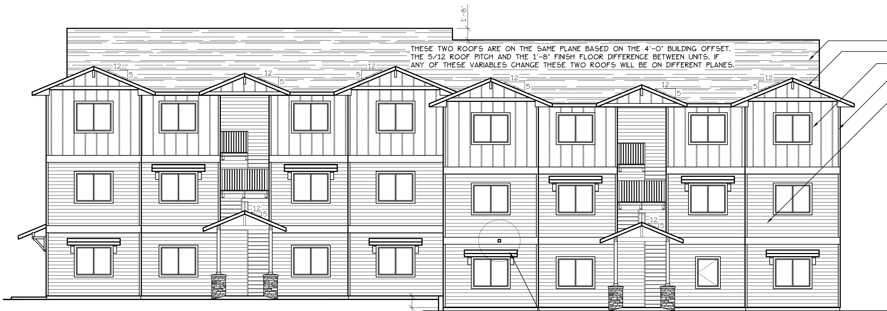
SOUTH ELEVATION (TYPE C UNITS) SCALE: 1/8" = 1'-0" BLD. 2
