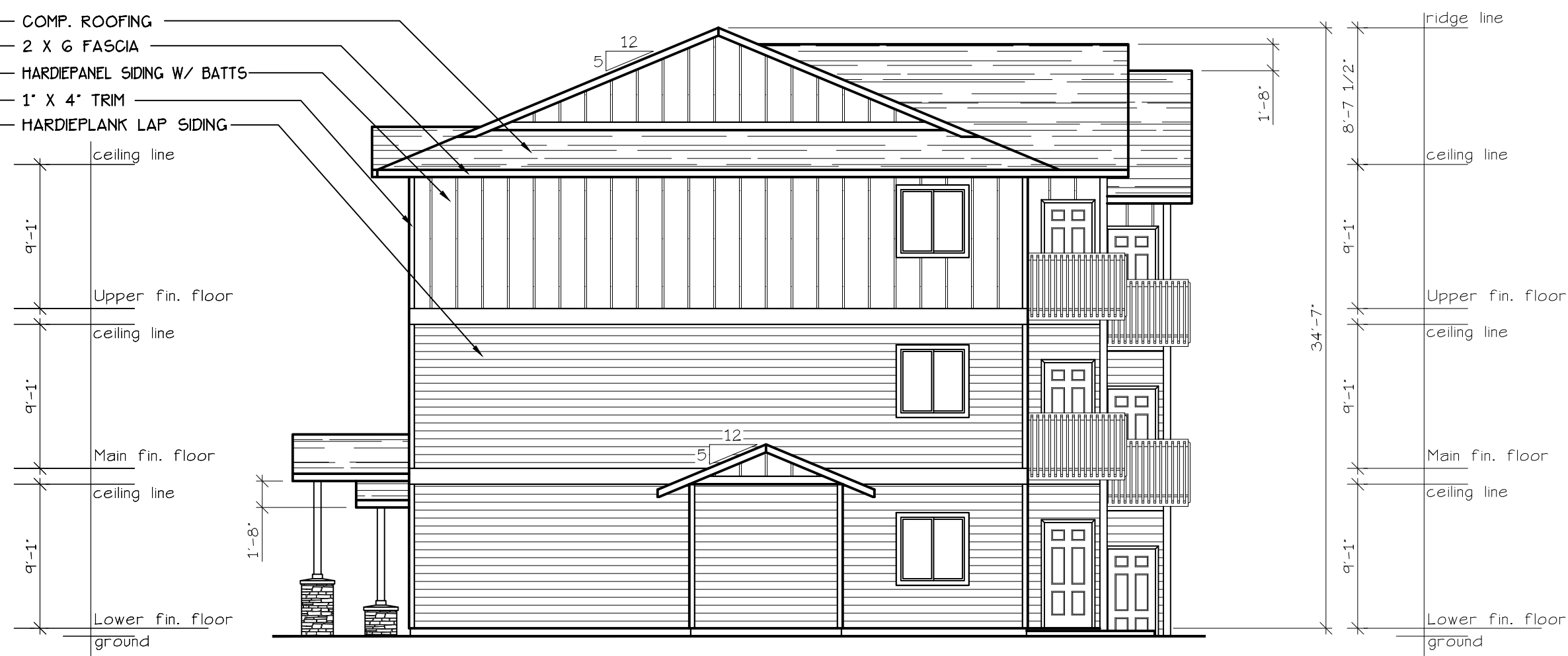
SOUTH ELEVATION (TYPE D UNITS) SCALE: 1/8" = 1'-0" BLD. 5
