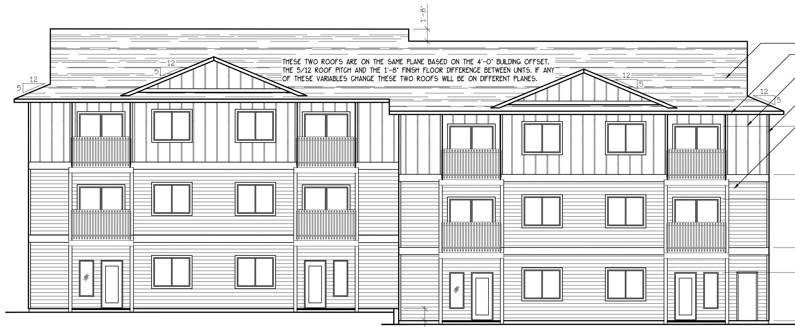
EAST ELEVATION (TYPE B UNITS) SCALE: 1/8" = 1'-0" BLD. 4
