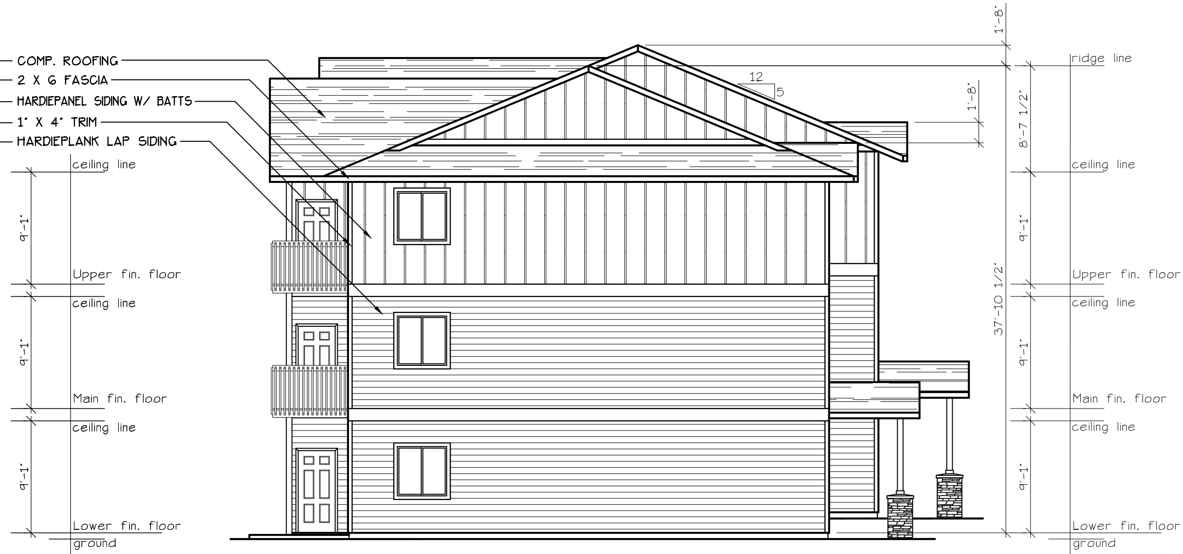
NORTH ELEVATION (TYPE D UNITS) SCALE: 1/8" = 1'-0" BLD. 5
